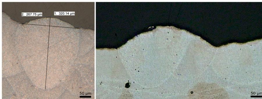
**Figure 3.** The two examined types of laser tracks. **Left:** *Primary track.* **Right:** *Secondary track.*
