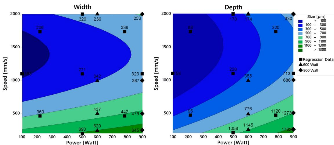
Figure 6. Melt pool width and depth for primary laser tracks. Topographical representation is based on the regression data. Data points of the full factorial design, which were used for the regression, are marked by squares. Data points of the single parameter variations marked by triangles and rhombs.
