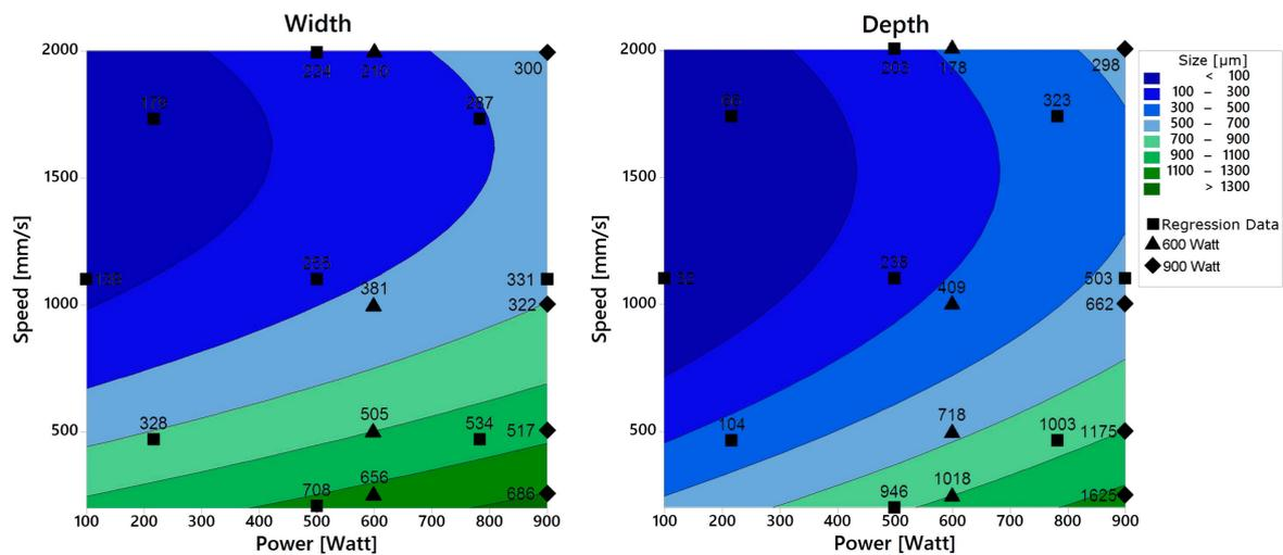
**Figure 7.** Melt pool width and depth for *secondary laser tracks*. Topographical representation based on the regression data. Data points of the full factorial design, which were used for the regression, are marked by squares. Data points of the single parameter variations marked by triangles and rhombs.
