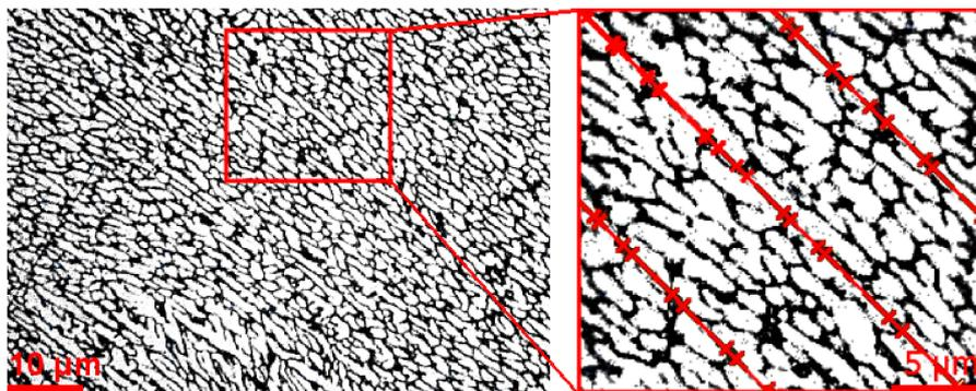
**Figure 4.** Linear intercept method used on binarized images under a magnification of 150 $\times$ .
