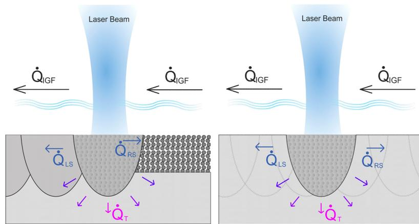
**Figure 2.** The two examined cases under different thermal boundary conditions. **Left:** *Primary laser track.* Illustrating the first exposure and melting of powder particles covering one layer thickness of 90  $\mu\text{m}$ . **Right:** *Secondary laser track.* Illustrating the re-exposure of already-created dense material.
