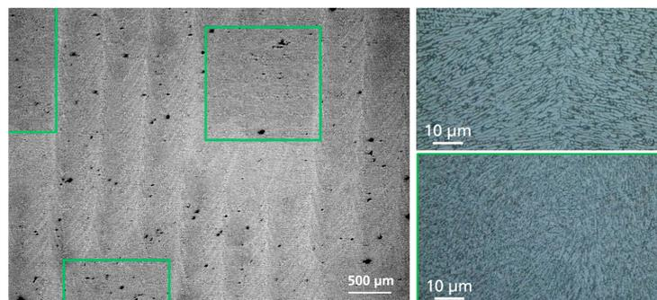
**Figure 9.** Application of results. Designed Material consisting of coarse- (top right) and fine-grained areas (bottom right marked in green).
