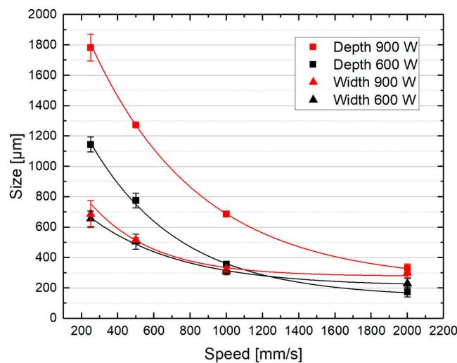
Figure 5. Melt pool dimensions for single parameter variation using secondary laser tracks.
