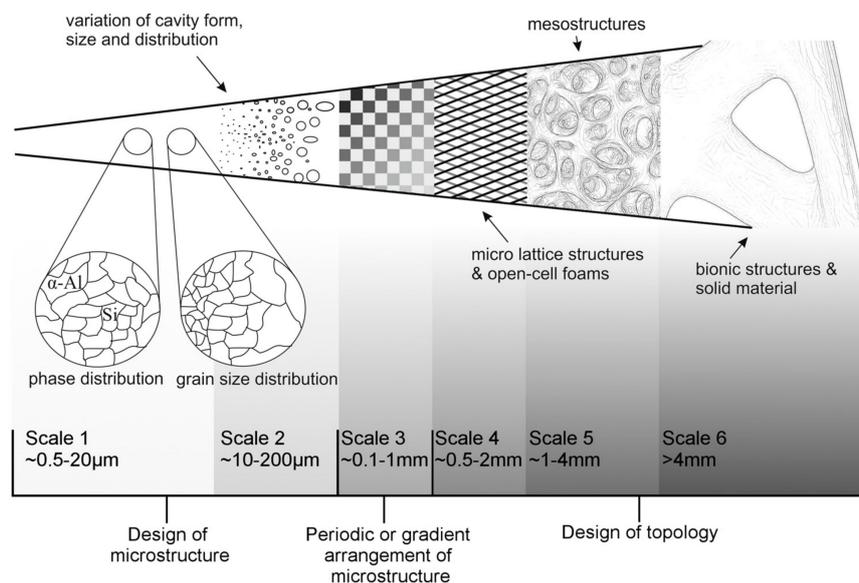
**Figure 1.** Proposed levels of influence to create a Designed Material. Based on these approaches, a material can be designed and optimized for a specific purpose or demand.
