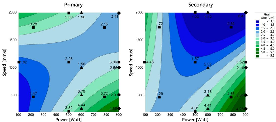
**Figure 8.** Grain length of Al phase for *primary* and *secondary laser tracks*. Topographical representation based on the regression data.
