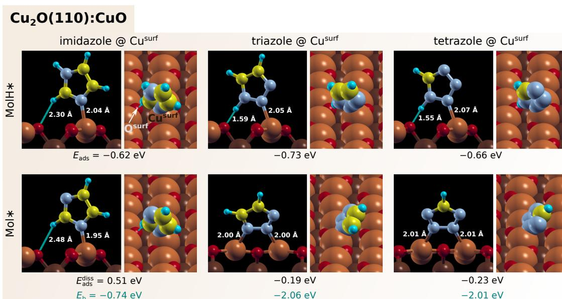
**Figure 7.** As in Figure 4, but for bonding at the Cu<sup>surf</sup> site of Cu<sub>2</sub>O(110):CuO. The calculations were performed with one molecule per ( $\frac{2}{0} \frac{1}{2}$ ) supercell; see also the top-view in Figure 3d.
