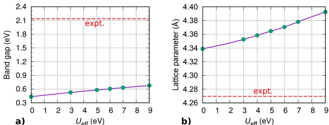
**Figure A1.** Effect of Hubbard  $U_{\text{eff}}$  parameter (applied to Cu  $d$  orbitals) on (a) band gap and (b) lattice parameter of  $\text{Cu}_2\text{O}$  bulk. Experimental values are also given (red-dashed line).
