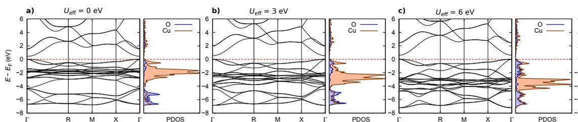
**Figure A2.** Effect of Hubbard  $U_{\text{eff}}$  parameter (applied to Cu  $d$  orbitals) on band structure and density of states of  $\text{Cu}_2\text{O}$  bulk projected (PDOS) onto Cu and O ions. The top of the valence band is chosen as the zero energy.
