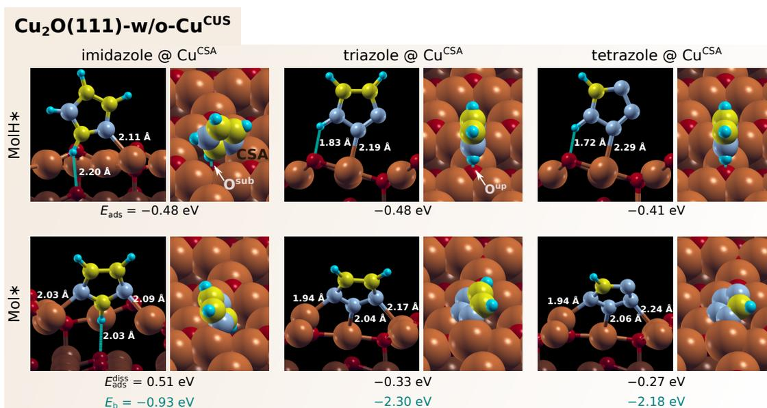
**Figure 5.** As in Figure 4, but for bonding at the Cu<sup>CSA</sup> site of Cu<sub>2</sub>O(111)-w/o-Cu<sup>CUS</sup>. The calculations were performed with one molecule per (2 × 2) supercell; see also the top-view in Figure 3b.
