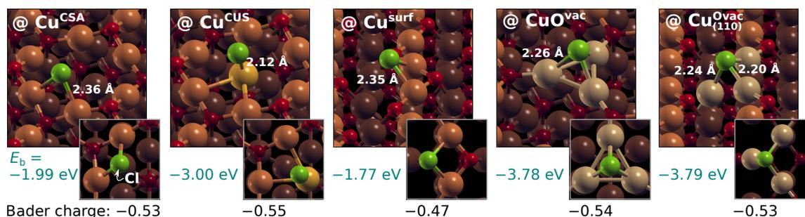
**Figure 16.** Snapshots of optimized structures of Cl\* (green balls) at various Cu sites on Cu<sub>2</sub>O surfaces; larger images show the perspective view and smaller images depict the top view. Cl\* binding energies and Bader charges as well as Cl–Cu bond-lengths are also given. The same supercells were used as for adsorption of azole molecules, cf. Figure 3.
