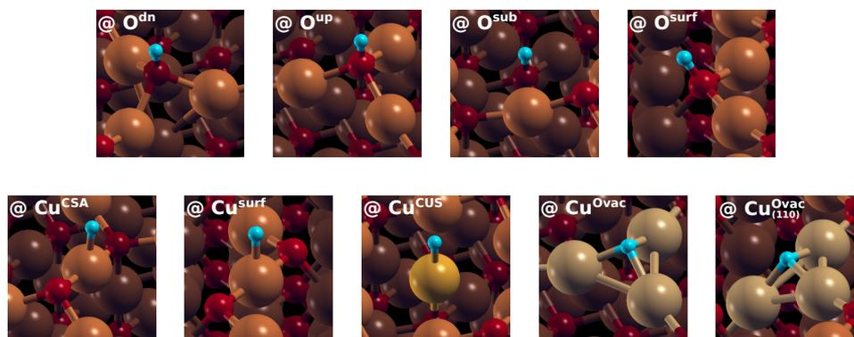
**Figure 13.** Snapshots of optimized structures of H adsorbed at various O (top row) and Cu (bottom row) sites on  $\text{Cu}_2\text{O}$  surfaces. Note that, upon adsorption of H onto  $\text{O}^{\text{dn}}$  site, the  $\text{O}^{\text{dn}}$  shifts upwards above the plane of surface  $\text{Cu}^{\text{CSA}}$  ions; hence, the  $\text{H} @ \text{O}^{\text{dn}}$  appears visually similar to  $\text{H} @ \text{O}^{\text{up}}$ .
