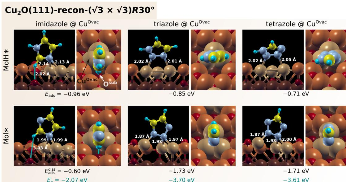
**Figure 6.** As in Figure 4, but for bonding at the Cu<sup>Ovac</sup> site of Cu<sub>2</sub>O(111)-recon-( $\sqrt{3} \times \sqrt{3}$ )R30°. The calculations were performed with one molecule per ( $\sqrt{3} \times \sqrt{3}$ )R30° unit cell; see also the top-view in Figure 3c.
