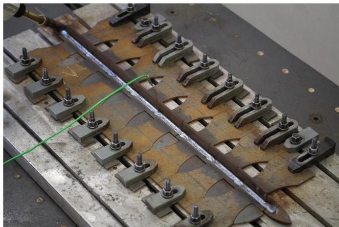
**Figure 1.** Overview of weld setup including  $t_{8/5}$ -measurement.
