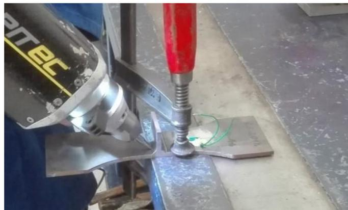
Figure 4. Clamping condition for HFMI-treatment.
