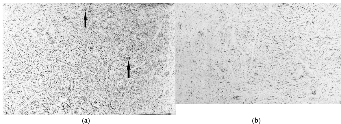
Figure 3. (a) Cross section of macro etched as cast unsoaked sample of alloy1. A-segregation channels are marked with arrows. Equiaxed crystals are visible. (b) Cross section of macro etched, as-cast soaked sample for 20 h, alloy1. Dendritic structure is not clearly visible due to homogenization of solute elements.
