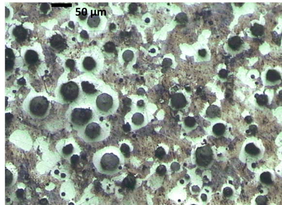
Figure 2. Microstructure of As-Cast Ductile Iron using Optical Microscopy at 100 \times .
