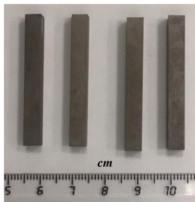
**Figure 7.** Pulsed electrospark deposition (PED) electrodes obtained using force self-propagating high-temperature synthesis (SHS)-pressing technology in a Ti–C–Co–Ca<sub>3</sub>(PO<sub>4</sub>)<sub>2</sub>–Ag–Mg system.
