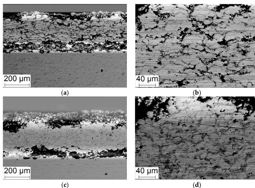
**Figure 4.** SEM-micrographs of the coating cross-section of specimens produced in regime No. 3 (a,b) and No. 4 (c,d).
