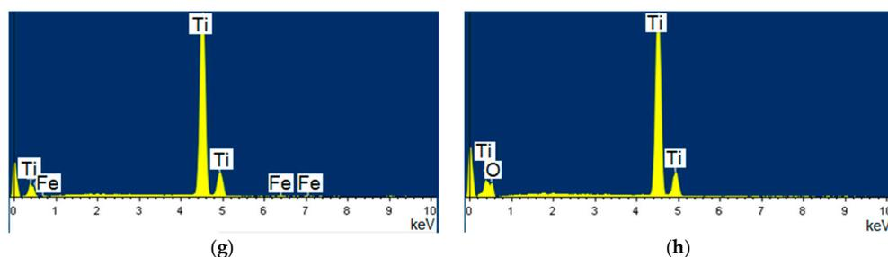
**Figure 3.** Micrographs of the coating cross-section and Energy Dispersive Spectroscopy (EDS) results: specimen produced in regime No. 1 (a–d) and No. 2 (e–h). A circle within red rectangle shows the location where EDS analysis was carried out.
