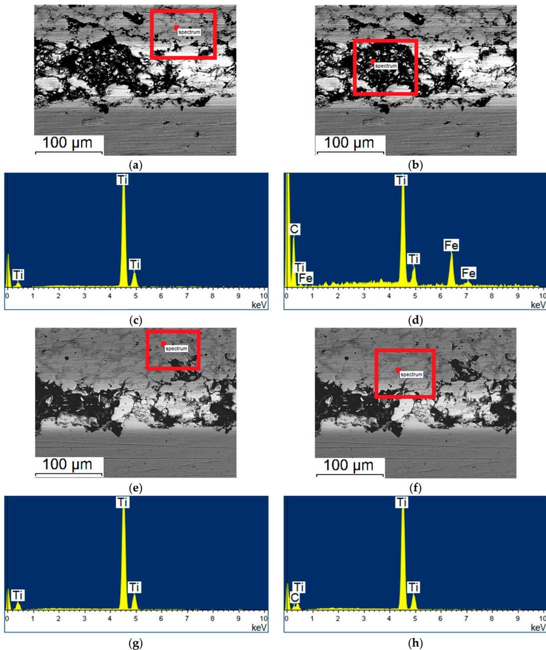
**Figure 5.** Micrographs of the coating cross-section and EDS results: specimen produced in regime No. 3 (a–d) and No. 4 (e–h). A circle within red rectangle shows the location where EDS analysis was carried out.
