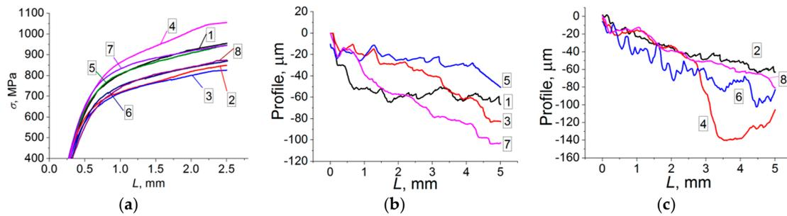
**Figure 1.** (a) three-point bending diagram for coated titanium specimens; (b,c) scratching diagrams of the coatings.
