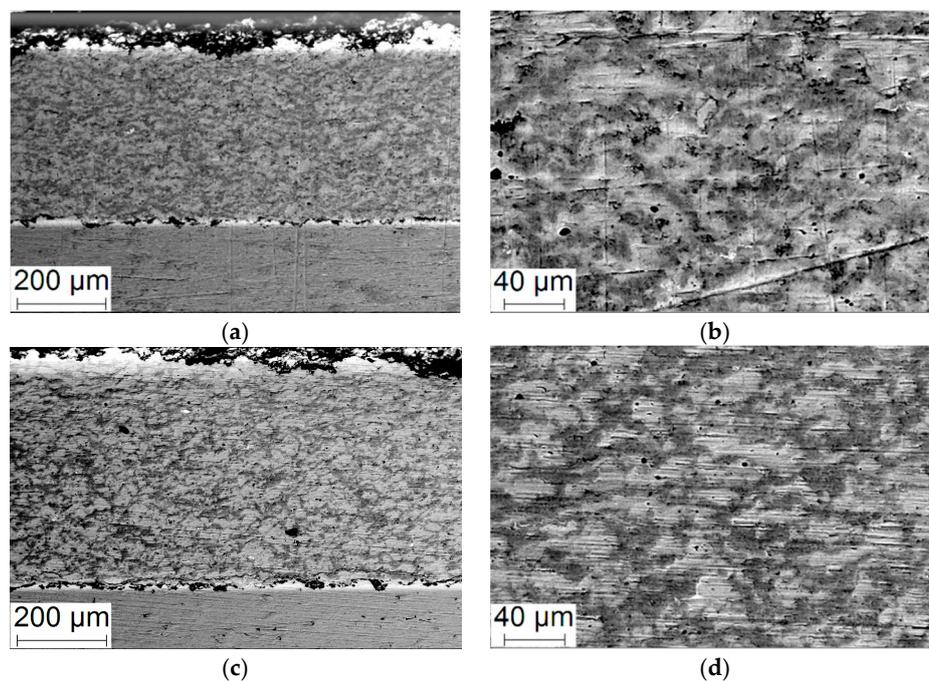
**Figure 6.** SEM-micrographs taken at the cross section of the specimens produced in regime No. 5 (a,b) and No. 6 (c,d).
