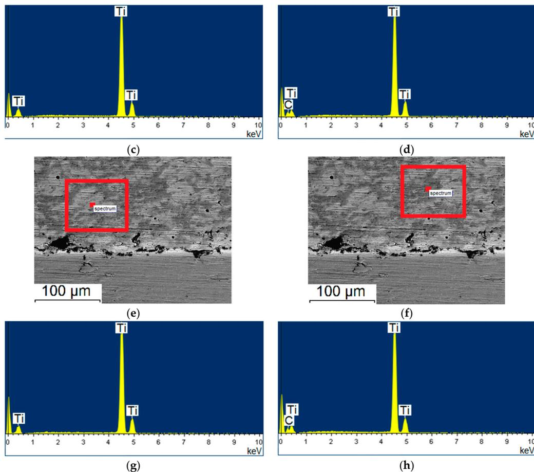
**Figure 7.** SEM-micrographs of the coating cross-section and EDS results: specimen produced in regime No. 5 (a–d) and No. 6 (e–h). A circle within red rectangle shows the location where EDS analysis was carried out
