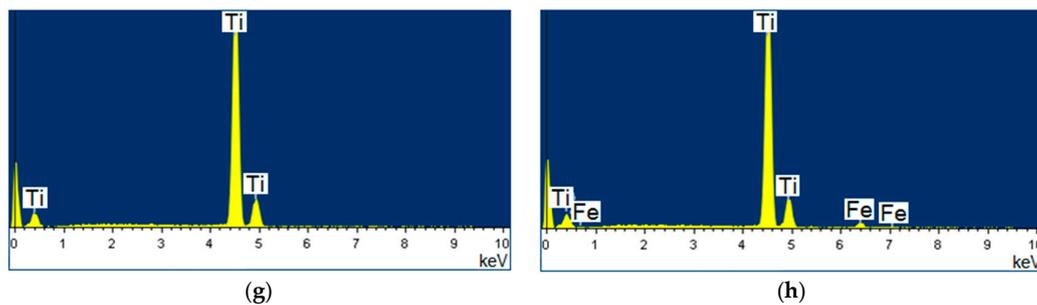
**Figure 9.** Micrographs of the coating cross-section and EDS results: specimen produced in regime No. 7 (a–d) and No. 8 (e–h). A circle within red rectangle shows the location where EDS analysis was carried out.
