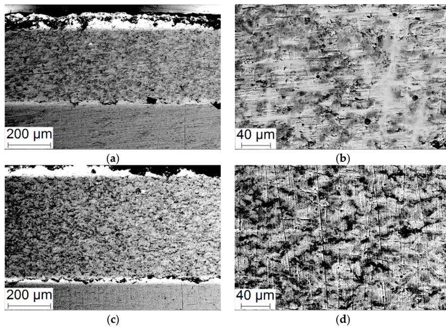
Figure 8. EM micrographs of the cross sections of specimens produced in regime No. 7 (a,b) and No. 8 (c,d).
