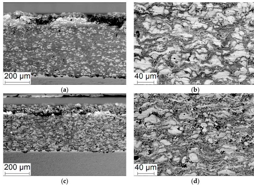
**Figure 2.** Scanning electron microscope (SEM)-micrographs of the cross section of specimens produced in regime No. 1 (a,b) and No. 2 (c,d).
