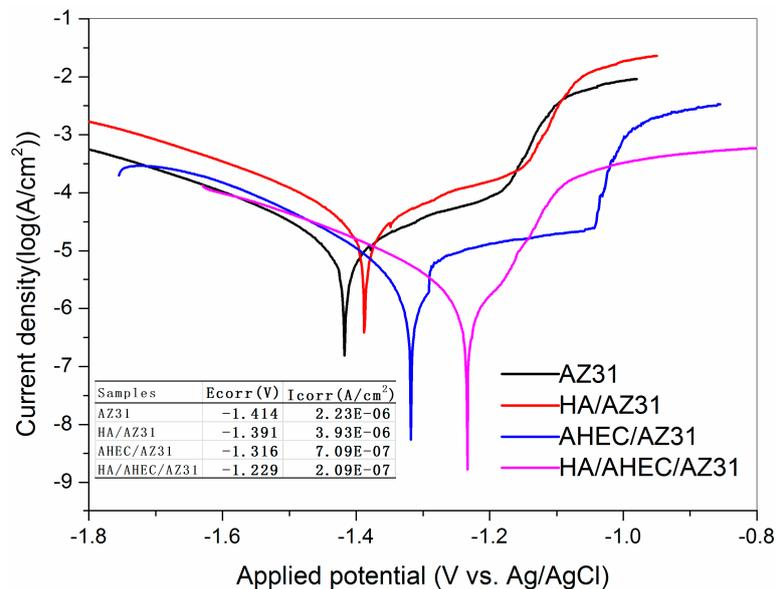
**Figure 4.** The potentiodynamic polarization curves for AZ31, HA/AZ31, AHEC/AZ31, and HA/AHEC/AZ31 in SBF at room temperature; the relative electrochemical parameters are listed in the inset.
