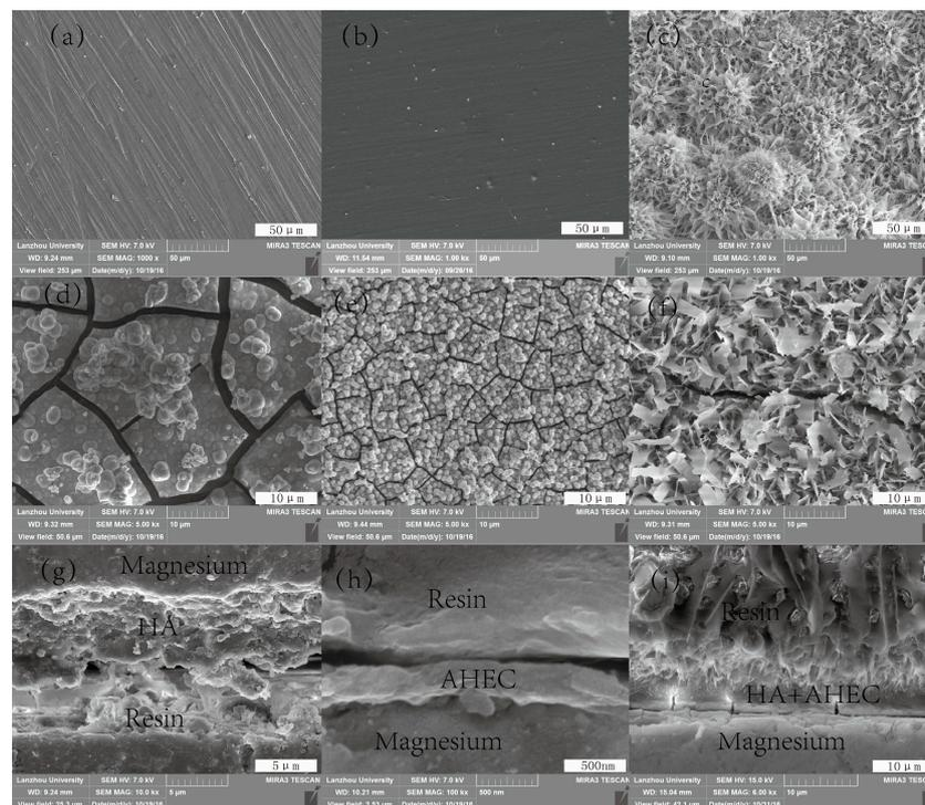
**Figure 1.** Scanning electron microscopy (SEM) images of AZ31, aminated hydroxyethyl cellulose (AHEC)/AZ31, and hydroxyapatite/aminated hydroxyethyl cellulose (HA/AHEC)/AZ31 specimens: before (a–c); and after (d–f) immersion in simulated body fluid (SBF) for 7 days; and the cross-sections of: (g) HA/AZ31; (h) AHEC/AZ31; and (i) HA/AHEC/AZ31.
