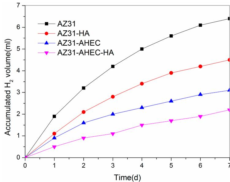
**Figure 6.** The line chart of cumulative hydrogen gas for the uncoated and coated samples in SBF for seven days.
