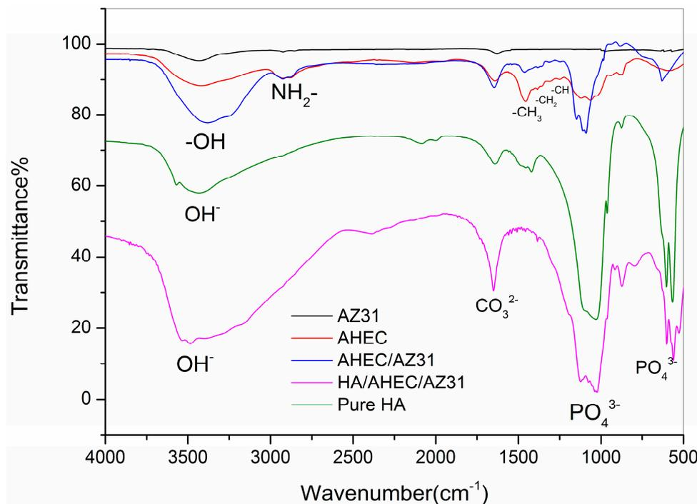
**Figure 3.** Fourier-transform infrared (FT-IR) spectrum of AZ31, AHEC, AHEC/AZ31, HA/AHEC/AZ31, and Pure HA.
