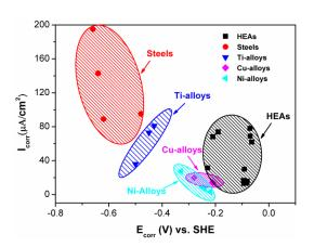
**Figure 5.** A comparison of the corrosion current density ( $i_{corr}$ ) and corrosion potential ( $E_{corr}$ ) between HEAs and conventional alloys in the 0.5 M H<sub>2</sub>SO<sub>4</sub> solution at room temperature.
