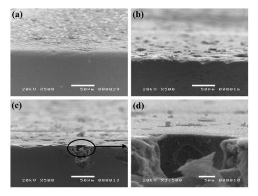
**Figure 3.** SEM micrographs for the  $Al_xCrFe_{1.5}MnNi_{0.5}$  alloys with varying amounts of aluminum content (**a**) x = 0; (**b**) x = 0.3 mol, (**c**) x = 0.5 mol; (**d**) higher magnification of micrograph (**c**) after anodic polarization exceeded the breakdown potential (>1.25 V<sub>SHE</sub>) in 0.5 M H<sub>2</sub>SO<sub>4</sub> [41] (Reprinted with permission from Elsevier).
