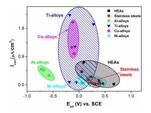
**Figure 4.** A comparison of the corrosion current density ( $i_{corr}$ ) and pitting potential ( $E_{pit}$ ) between HEAs and other materials in the 3.5 wt % NaCl solution at room temperature.
