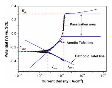
**Figure 1.** A typical potentiodynamic-polarization curve for the explanation of the parameters.  $E_{\text{corr}}$ , corrosion potential;  $i_{\text{corr}}$ , corrosion current density; Passivation area, the potential range where a protective oxide film formed to prevent the continual metal from dissolving;  $E_{\text{pit}}$ , critical pitting potential;  $i_{\text{pass}}$ , current density in the passivation area.
