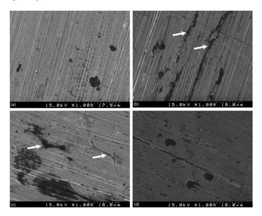
**Figure 2.** The surface appearance of alloys after immersion tests in the 3.5 wt % NaCl solution for 30 days: (a) FeCoNiCr; (b) FeCoNiCrCu<sub>0.5</sub>; (c) FeCoNiCrCu; and (d) 304 L (white arrows point to the localized corrosion caused by electrochemical attack along the interdendrites) [44] (Reprinted with permission from Elsevier).
