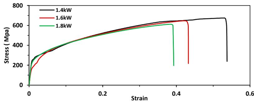
Figure 18. Typical trend of the 2205-304 in stress-strain diagram.
