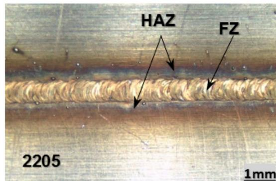
Figure 7. Plan view of the seam welding.
