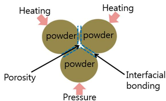
**Figure 3.** Schematic of sintering process.
