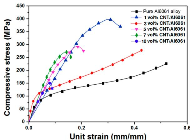
**Figure 6.** Compressive stress-strain curve of each material (compaction pressure: 1 GPa; sintering temperature: 620 °C).
