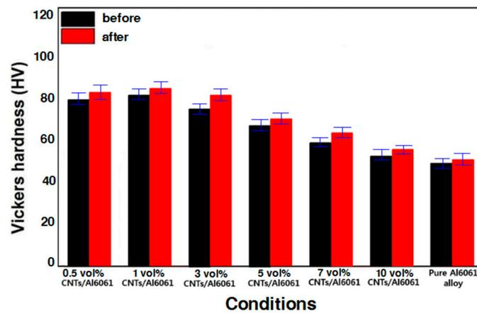
**Figure 5.** Vickers hardness of cross sections in the direction of compaction before and after sintering (compaction pressure: 1 GPa; sintering temperature: 620 °C).
