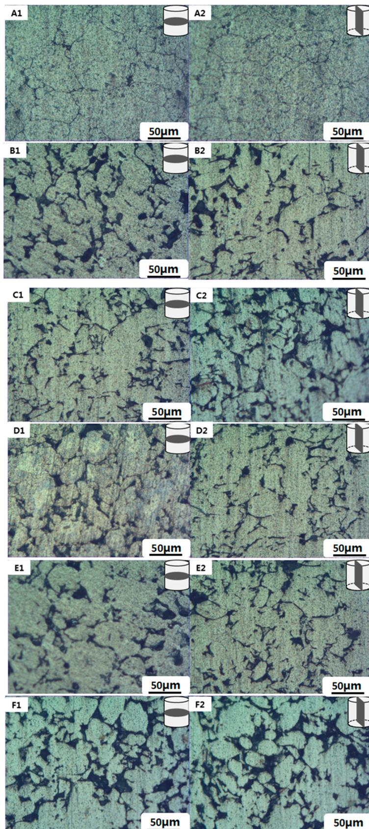
**Figure 8.** Microstructure for variation of MWCNTs volume fraction before open-die forging ((A1,A2) Al6061; (B1,B2) 1 vol %; (C1,C2) 3 vol %; (D1,D2) 5 vol %; (E1,E2) 7 vol %; (F1,F2) 10 vol %).
