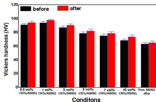
Figure 9. Vickers hardness in the direction of compaction after open-die forging.
