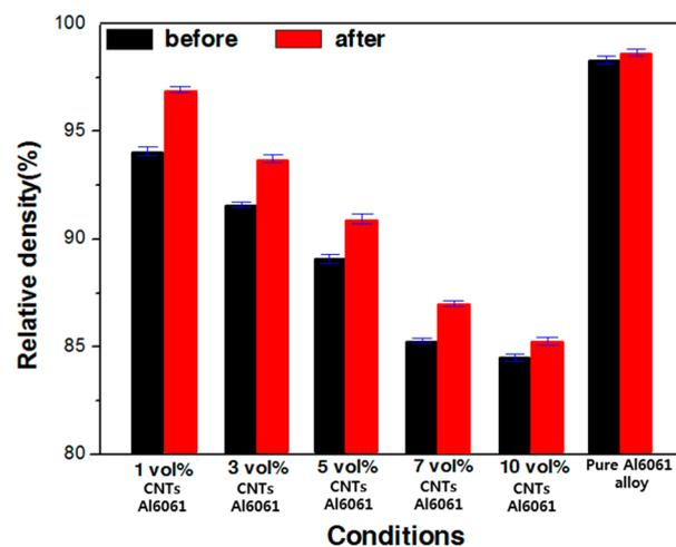
**Figure 7.** Change phenomenon of relative density before and after open-die forging (compaction pressure: 1 GPa; sintering temperature: 620 °C).
