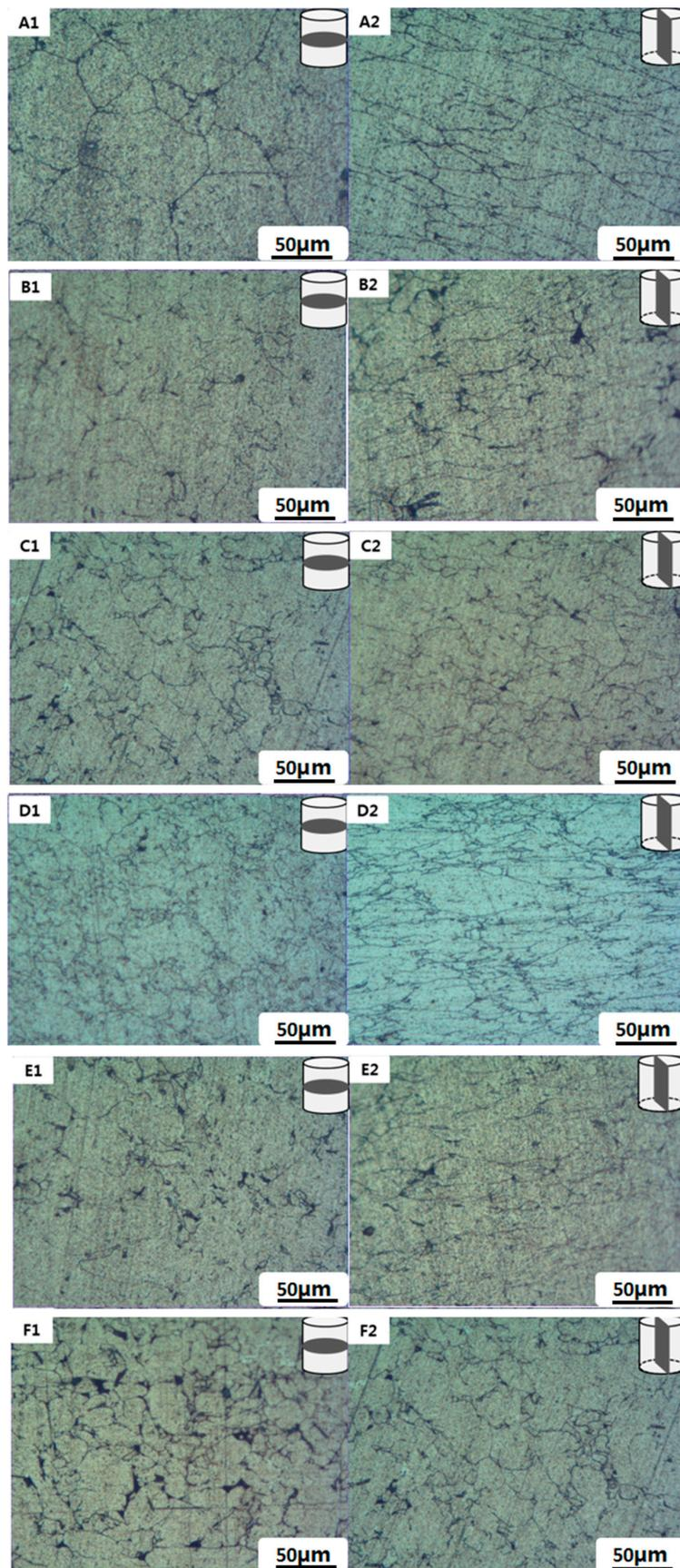
**Figure 10.** Microstructure for variation of MWCNTs volume fraction after open-die forging ((A1,A2) Al6061; (B1,B2) 1 vol %; (C1,C2) 3 vol %; (D1,D2) 5 vol %; (E1,E2) 7 vol %; (F1,F2) 10 vol %).
