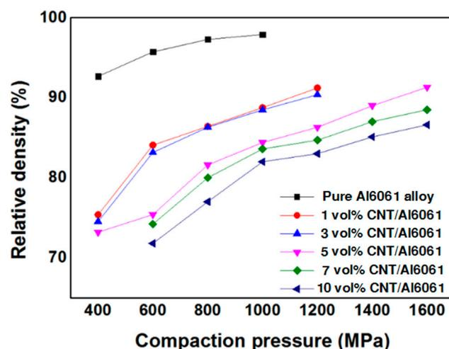
Figure 4. Change phenomenon in the relative density of each material depending on compaction pressure.
