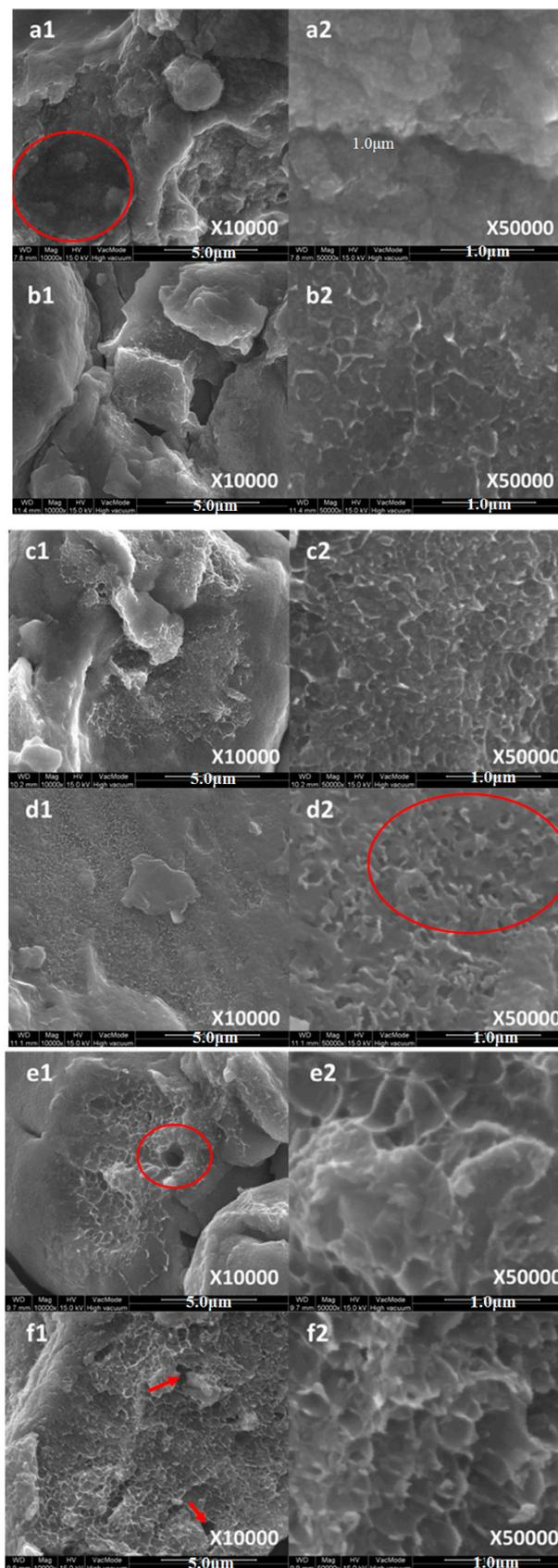
**Figure 11.** SEM micrographs of fracture cross section by low magnification and high magnification in (allow refer to dimple) ((a1,a2) Al6061; (b1,b2) 1 vol %; (c1,c2) 3 vol %; (d1,d2) 5 vol %; (e1,e2) 7 vol %, and; (f1,f2) 10 vol %).
