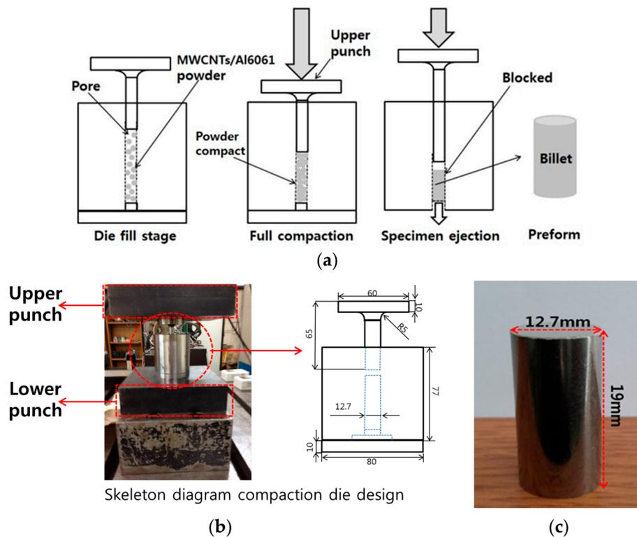
**Figure 2.** (a) Cold-compaction process; (b) equipment (unit: mm); and (c) billet.
