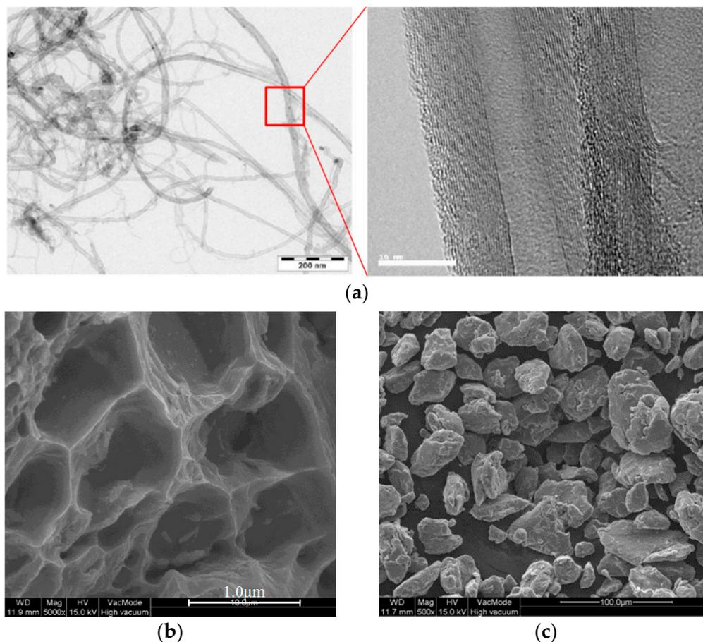
**Figure 1.** (a) Transmission electron microscopy (TEM) micrographs of pristine multi-walled carbon nanotubes (red square : 20 times magnification); (b) scanning electron microscopy (SEM) images of Al6061 and (c) SEM images of MWCNTs mixture powder.
