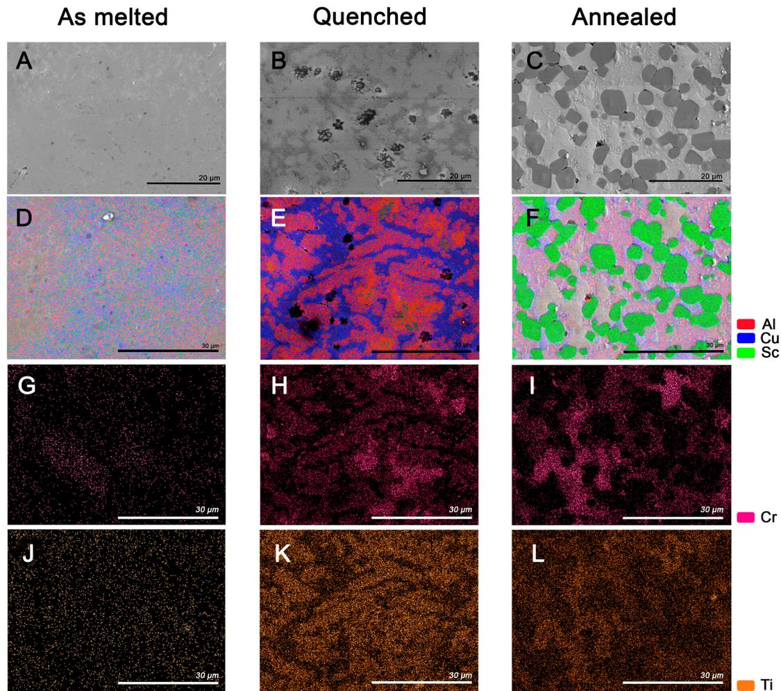
**Figure 2.** SEM images of as melted (A), quenched (B) and annealed (C) AlCrCuScTi alloy. EDX elemental composition maps of Al, Cu and Sc for as melted (D), quenched (E) and annealed (F) AlCrCuScTi alloy respectively. EDX elemental composition maps of Cr distribution for as melted (G), quenched (H) and annealed (I) AlCrCuScTi alloy respectively. EDX elemental composition maps of Ti distribution for as melted (J), quenched (K) and annealed (L) AlCrCuScTi alloy respectively.
