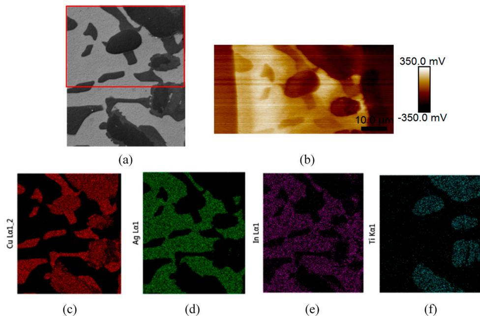
**Figure 9.** Secondary electron SEM image of Cu-Ag-In-Ti sample with the red box indicating where SKPFM was performed (a). SKPFM surface potential image (b) and EDS elemental maps of the identical region for: Copper (c); Silver (d); Indium (e); and Titanium (f) are shown.
