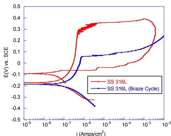
**Figure 6.** Potentiodynamic polarization scans conducted on 316L stainless steel subjected to a thermal brazing cycle (blue curve) compared to unfired 316L (red curve). Testing was conducted in 0.6 M NaCl with a scan rate 0.166 mV/s.
