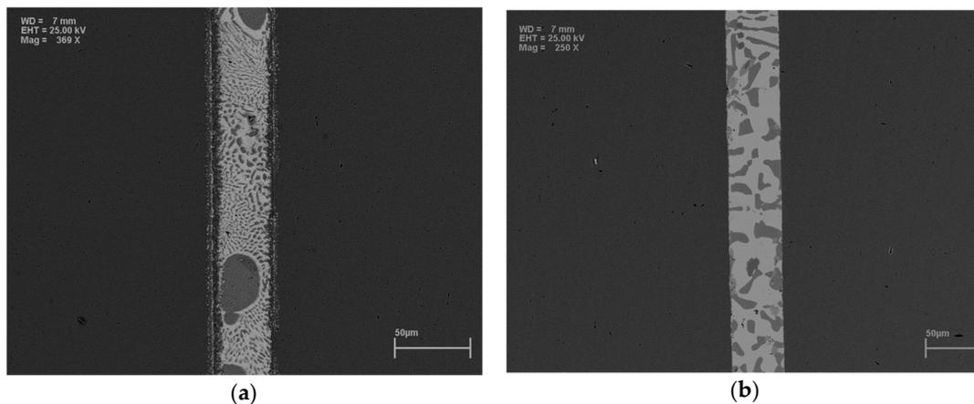
**Figure 1.** Scanning Electron Microscopy (SEM) images of cross sections of the resultant braze joint between two stainless steel 316L samples joined using: Cu-Ag-Ti (a) and Cu-Ag-In-Ti (b) braze alloys.
