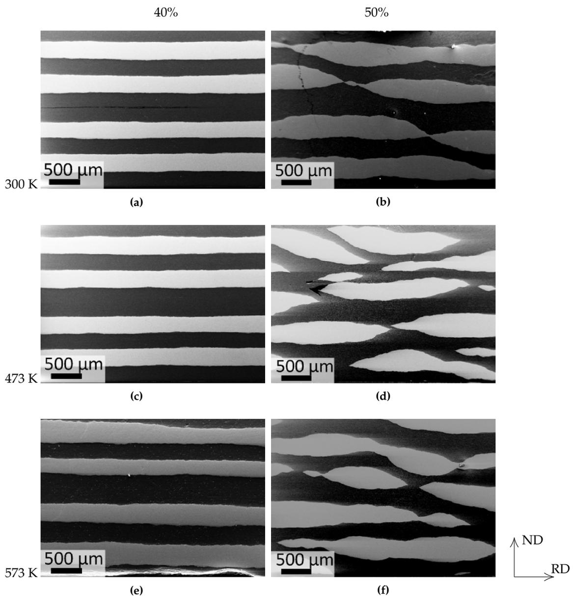
**Figure 9.** SEM micrographs showing the layer structure of a five-layered composite roll bonded with a single ARB cycle at elevated temperatures. The sheets are rolled with a 40% (a,c,e) or a 50% (b,d,f) thickness reduction during the second cycle.
