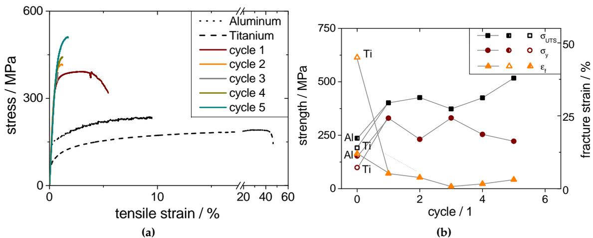
**Figure 3.** Engineering stress-strain curves of the five-layered Ti/Al composite accumulatively roll bonded with up to five cycles without intermediate heat treatments (a) and ultimate tensile strength ( $\sigma_{UTS}$ ), yield strength ( $\sigma_y$ ) and plastic strain ( $\epsilon$ ) of Al (half open symbols), Ti (open symbols) and the five-layered composite (filled symbols) (b).
