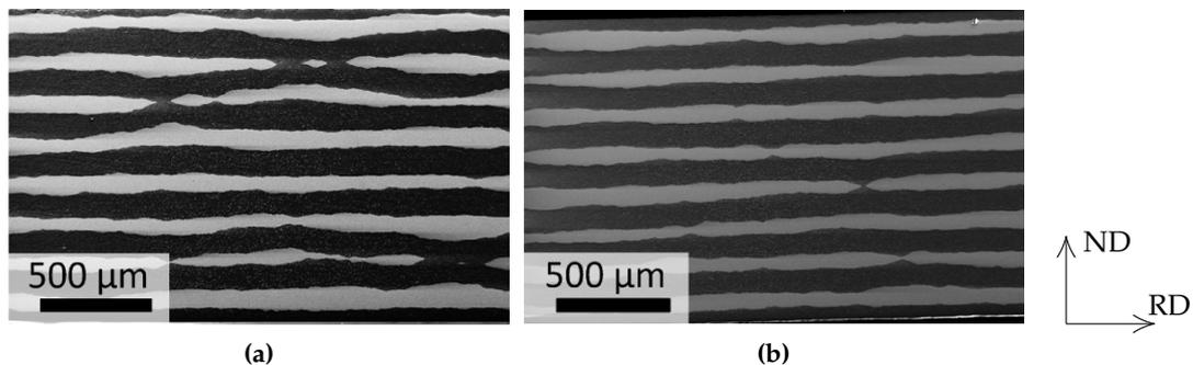
**Figure 10.** Cross-section of the layer structure after four ARB cycles in a trio (a) and four high rolling mill (b).
