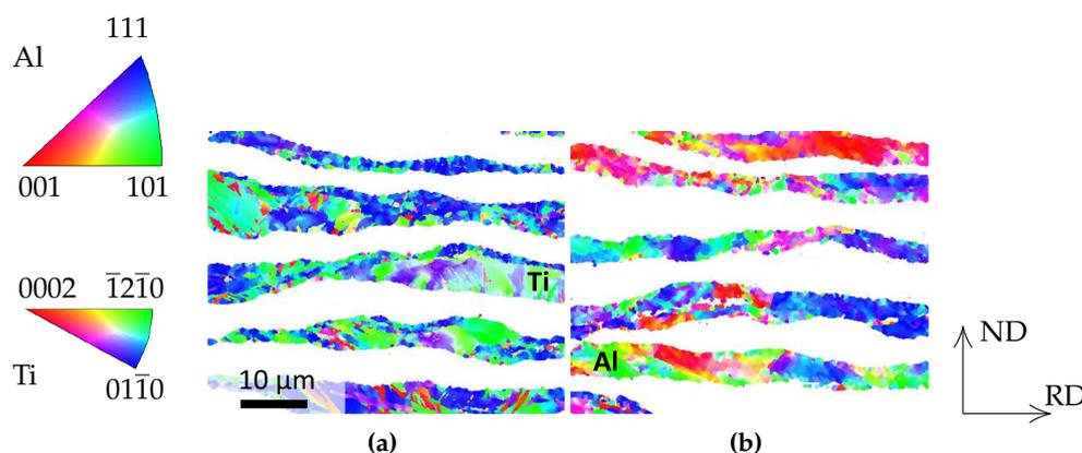
**Figure 8.** Electron backscatter diffraction (EBSD) maps of a five-layered composite sheet after eight ARB + IHT cycles. The maps are separated for Ti (a) and Al (b). The color code describes the crystal orientation in the rolling direction according to the inverse pole figure maps (shown leftmost for the cubic (Al, upper part) and hexagonal case (Ti, lower part)).
