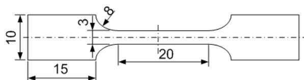
Figure 1. Geometry of the samples used for tensile tests. Dimensions are provided in mm.
