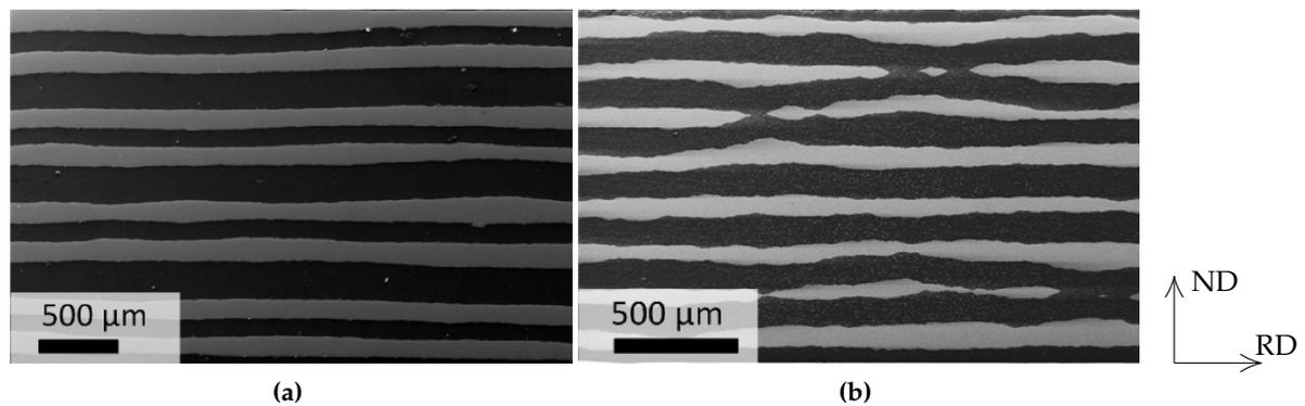
**Figure 7.** Micrographs showing the longitudinal sections of five-layered composites after four ARB cycles; rolling with a strain rate of  $23.4 \text{ s}^{-1}$  (a) and  $5.3 \text{ s}^{-1}$  (b).
