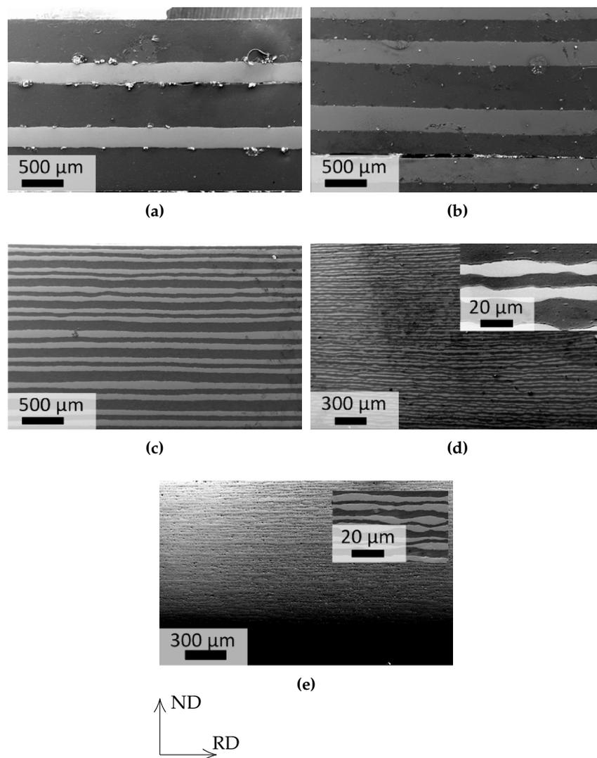
**Figure 4.** SEM micrographs showing the longitudinal cross-section of the layer structure of a Ti/Al composite sheets after accumulatively roll bonding a five-layered composite after the first (a), second (b); fourth (c), sixth (d) and eighth (e) ARB cycle with IHTs being applied.
