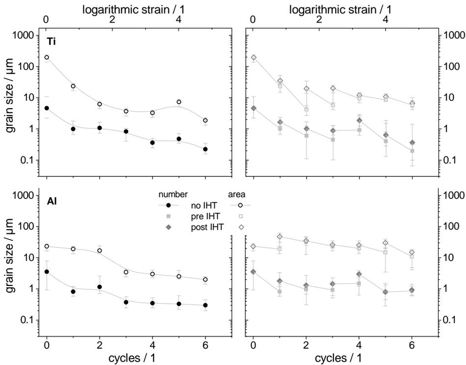
**Figure 5.** Grain size within the Ti (upper row) and Al layers (lower row) after ARB at room temperature (left), as well as with IHTs applied (right). In the latter case, the grain sizes are provided after the ARB cycles before (pre-IHT) and after IHT (post-IHT). The grain sizes were evaluated by both number and area weighting.
