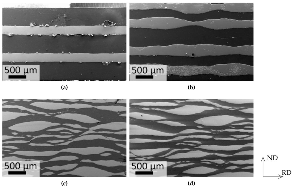
**Figure 2.** SEM micrographs showing the longitudinal cross-section of Ti/Al composite sheets after accumulative roll bonding a five-layered composite, *i.e.*, after the first (a), second (b), fourth (c) and sixth (d) accumulative roll bonding (ARB) cycle (no intermediate heat treatment (IHT) was applied).
