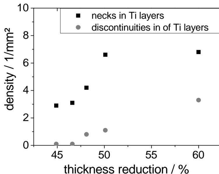
**Figure 11.** Density of necks and separated necks of a Ti/Al composite sheet after four ARB passes in a trio rolling mill in dependence of the thickness reduction during the last rolling cycle.
