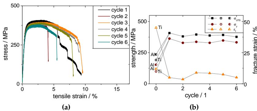
**Figure 6.** Engineering stress-strain curves of the five-layered Ti/Al composite accumulatively roll bonded with up to six cycles, including intermediate heat treatments (IHT) (a) and ultimate tensile strength ( $\sigma_{UTS}$ ), yield strength ( $\sigma_y$ ) and plastic strain ( $\epsilon$ ) of Al (half open symbols), Ti (open symbols) and the five-layered composite (filled symbols) (b).
