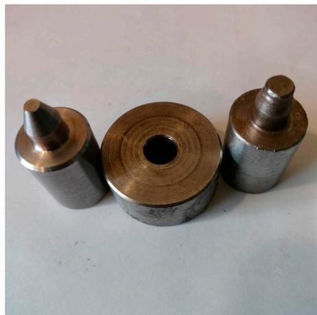
**Figure 3.** Die and punches used to create the gaps in the copper pipes.
