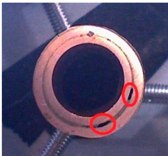
**Figure 13.** Example of a part that has failed the leakage test due to a lack of filler material.
