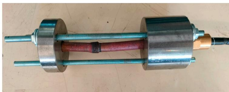
**Figure 8.** Tool for tightness testing of the samples.
