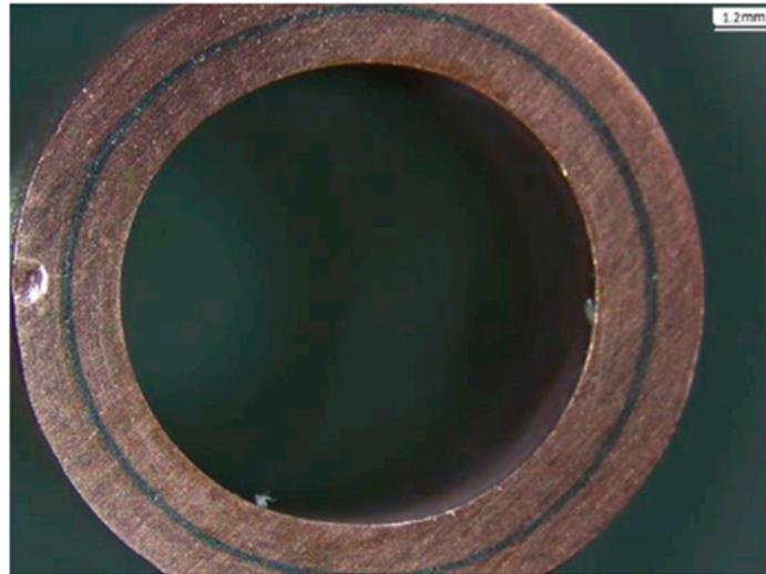
**Figure 10.** Stereo microscope image of the pipe cut transversely to the brazed connection.
