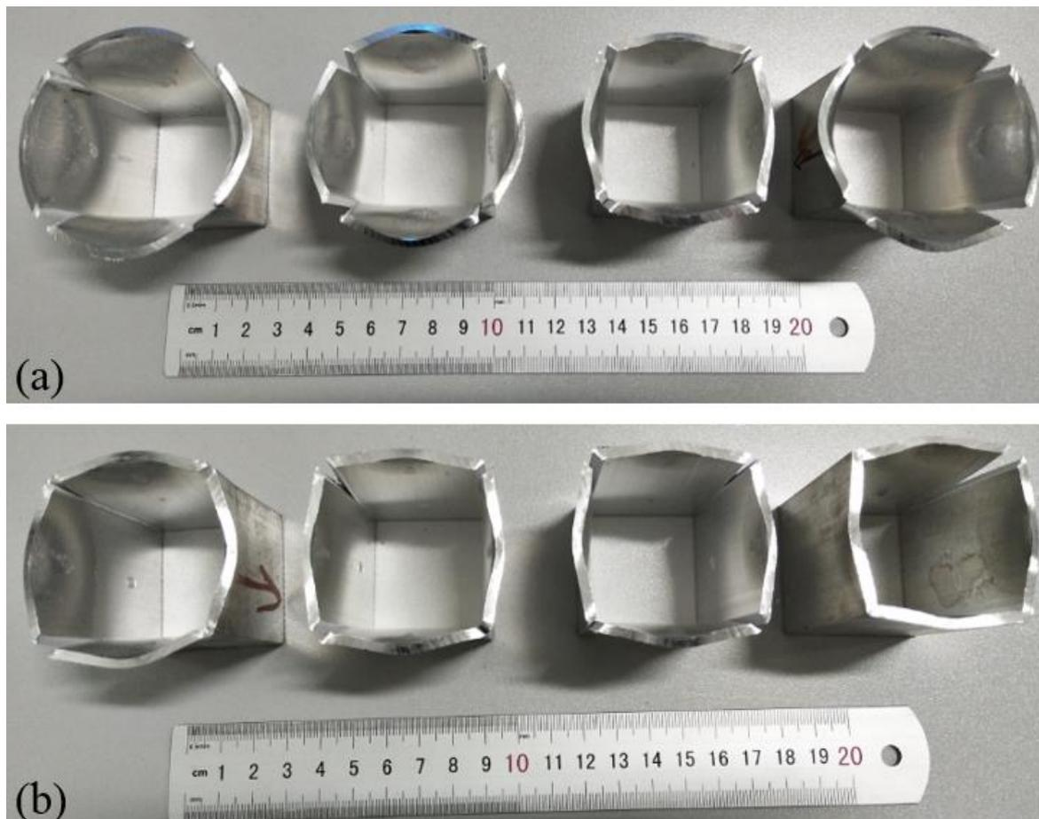
**Figure 12.** Macro-morphology of fracture after expanding test of PE11 with an aging time of (a) 2 h and (b) 8 h.
