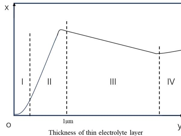
**Figure 1.** Corrosion rate at different liquid film thicknesses (The liquid film on the surface is divided into regions I–IV depending on the thickness of the liquid film) [7].
