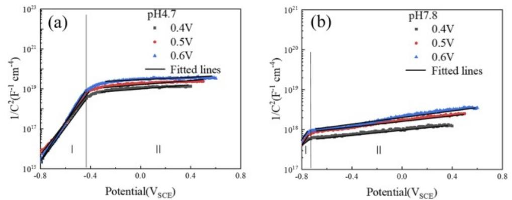
**Figure 5.** MS curves of solder Sn-0.7Cu in different environments (acidic (a) and alkaline (b) artificial sweat) [45].
