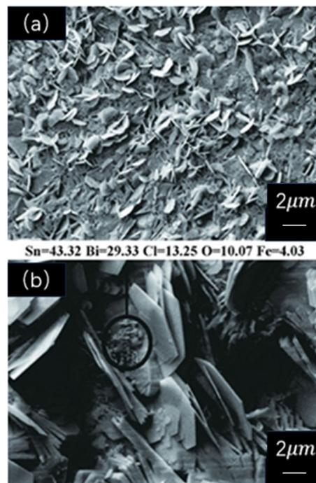
**Figure 3.** FESEM micrographs of solder alloys after complete polarization. (a) Sn–Cu; (b) Sn–Cu–Fe–1Bi [40].
