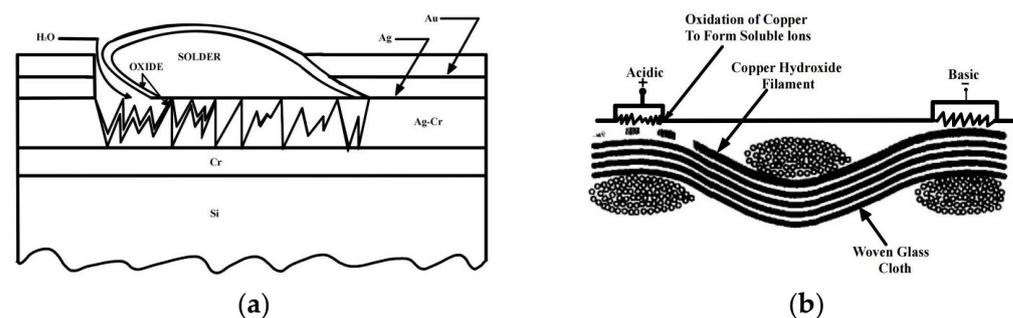
**Figure 2.** (a) Schematic diagram of the failure process at the chip chromium/solder interface [23]. (b) Schematic diagram of the cross-section of the printed chip circuit board [23].
