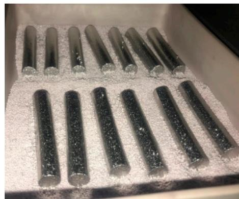
**Figure 5.** Sintered tensile test blanks.
