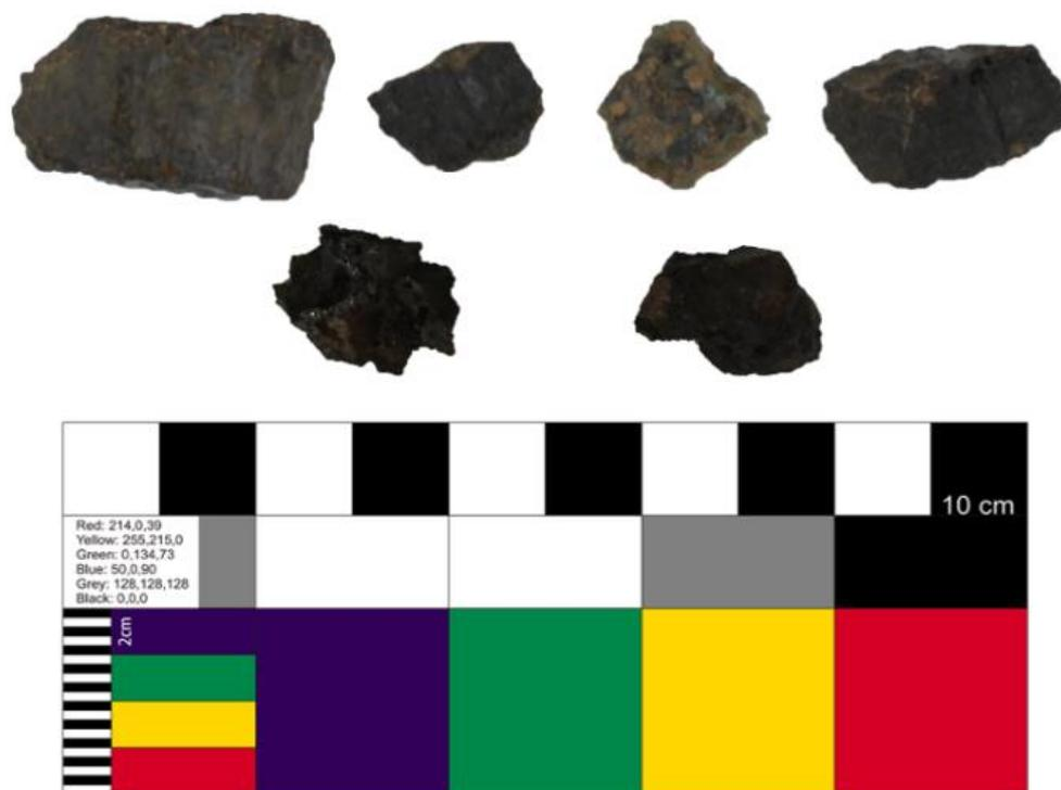
**Figure 5.** Appearance of slag samples from the Qingyuan site.
