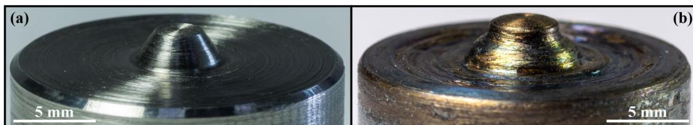
**Figure 22.** FSW tool produced from alloy ZhS6U before welding (a) and after  $\approx 0.5$  m of welding (b).
