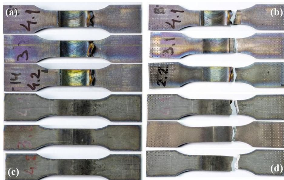
Figure 5. FSW joint tensile specimens of Ti-4Al-3Mo-1V titanium alloy: top view before (a) and after testing (b), and bottom view before (c) and after testing (d).
