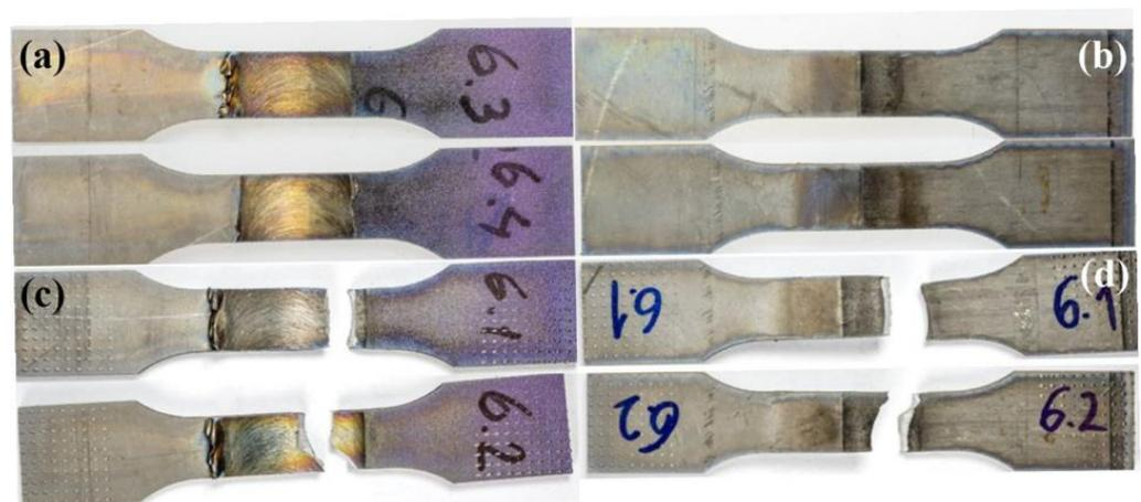
**Figure 9.** FSW joint tensile specimens of Ti-4Al-3Mo-1V/Ti-6Al-4V titanium alloys: top (a) and bottom view before testing (b), and top (c) and bottom view after testing (d).
