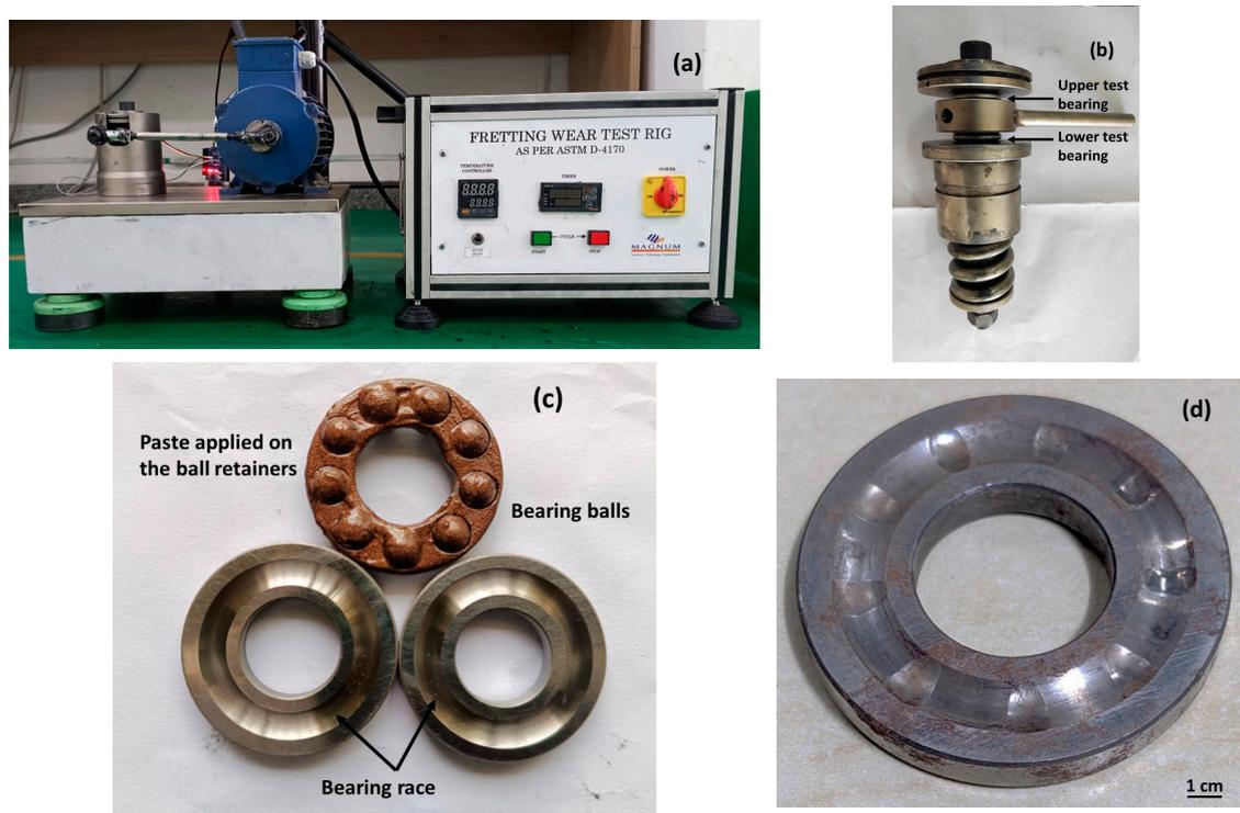
**Figure 2.** (a) Fafnir fretting wear test rig; (b) arrangement of the test bearings in the Fafnir test rig; (c) paste applied on the bearing race; and (d) false brinelling indentation marks on the bearing raceway after the fretting test.
