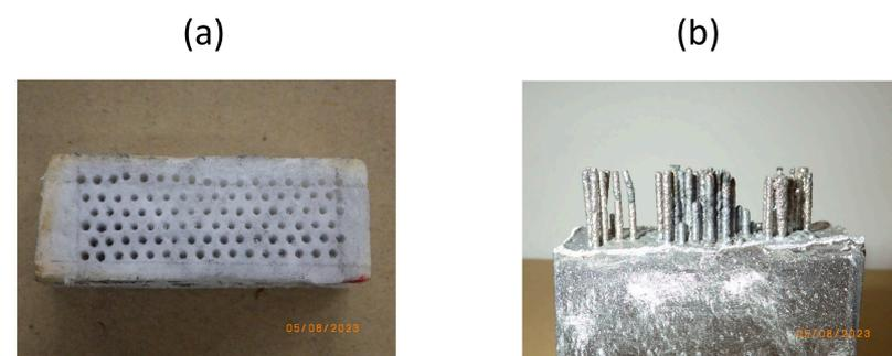
**Figure 9.** (a) Ninety-seven holes perforated by a micro-drill in a ceramic fiber block. Height of block: 15 mm; holes: 1.2 mm in diameter. (b) Only half of the columns were fabricated by casting, and others were not.
