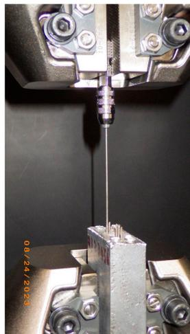
**Figure 12.** Extraction process of SUS wire coated with the mixture of disassembled fibers and polyvinyl alcohol. SUS wire: 0.97 mm in diameter and 75 mm in length.
