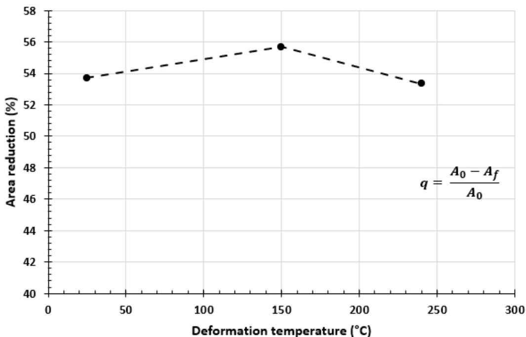
**Figure 11.** Contraction at fracture as measured and calculated from tensile specimens tested at 25, 150, and 240 °C.
