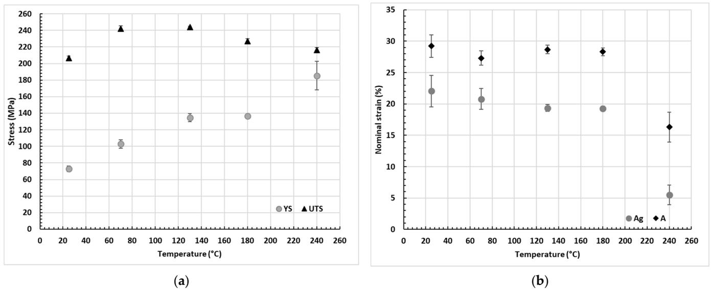
**Figure 5.** Resulting mechanical properties during warm tensile testing on specimens heated to different temperatures from W-temper are presented in (a) yield strength (YS) and ultimate tensile strength (UTS) as a function of deformation temperature and (b) total elongation (A) and elongation at maximum strength (Ag).
