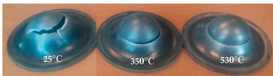
**Figure 8.** The force-displacement curve after formability cup testing of AA6082 at different conditions and temperatures with a displacement of 32 mm. Formed cups are shown in the lower image. From left to right: 25 °C, 350 °C, and 530 °C.
