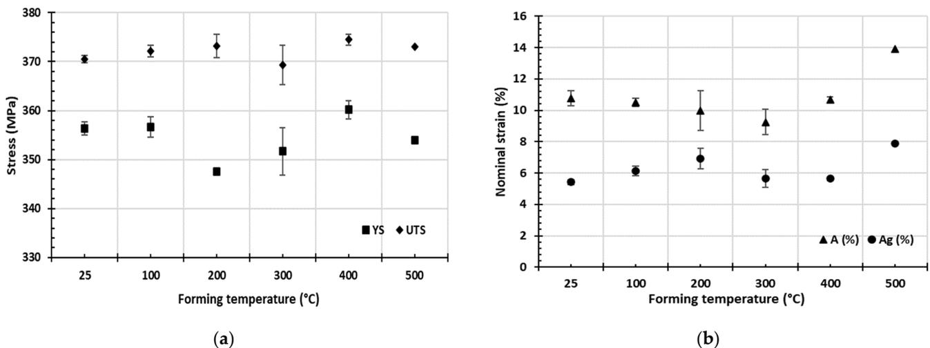
**Figure 2.** The resulting mechanical properties of AA6010 sheets after trials with different forming temperatures [6] are presented in (a) yield strength (YS) and ultimate tensile strength (UTS) as a function of deformation and (b) total elongation (A) and elongation at maximum strength (Ag).
