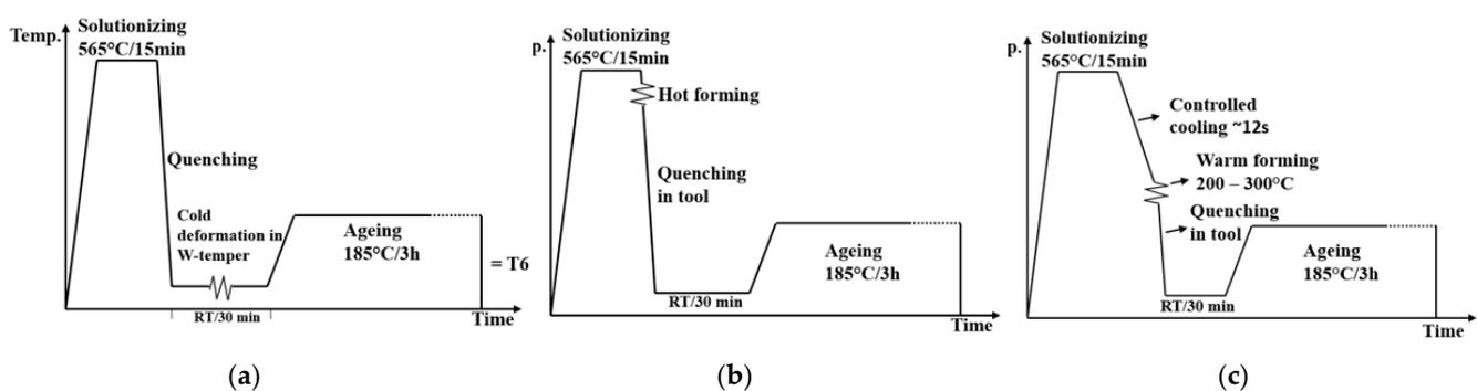
**Figure 1.** Illustrations of the thermomechanical process routes tested in previous research [5,6] where routes represent (a) cold forming, (b) hot forming, and (c) warm forming.
