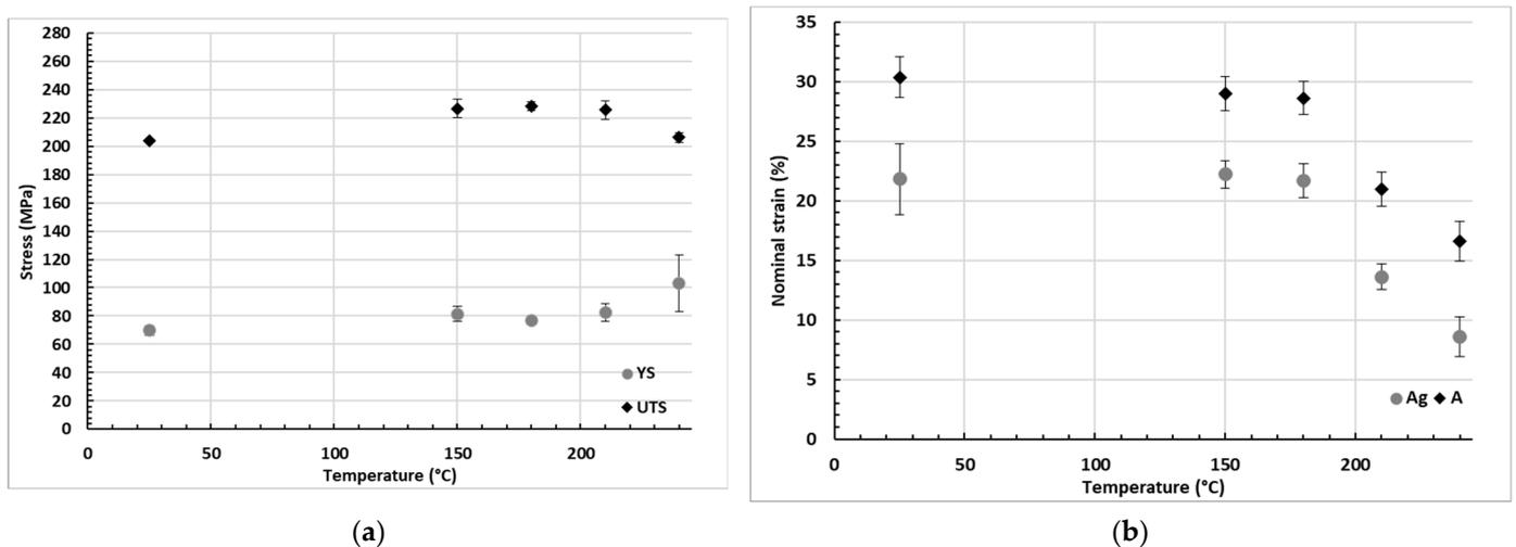
**Figure 6.** Resulting mechanical properties during warm tensile testing on specimens in W-temper, i.e., after cooling from SHT to target deformation temperature are presented by (a) yield strength (YS) and tensile strength (UTS) as a function of deformation temperature and (b) total elongation (A) and elongation at maximum strength (Ag).
