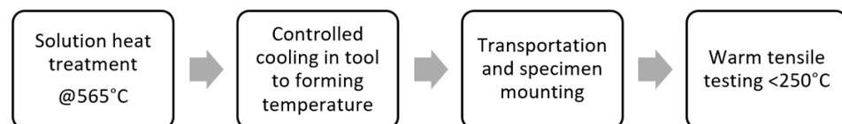
**Figure 3.** The test route developed for tensile tests in W-condition.
