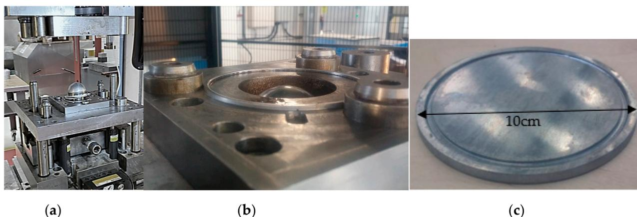
**Figure 4.** Formability cup tests, equipment, and samples. (a) The cup tool attached to a 300-ton press (b) the lower die with clamping ring to fix the blank during deep drawing, and (c) the blank with pre-formed grooves with a depth of 1.5–2 mm to fit the clamping ring.
