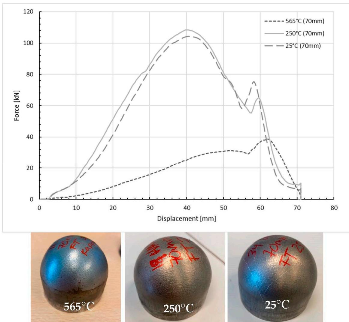
**Figure 7.** Force-displacement curve of samples formed at 565 °C, 250 °C, and 25 °C.
