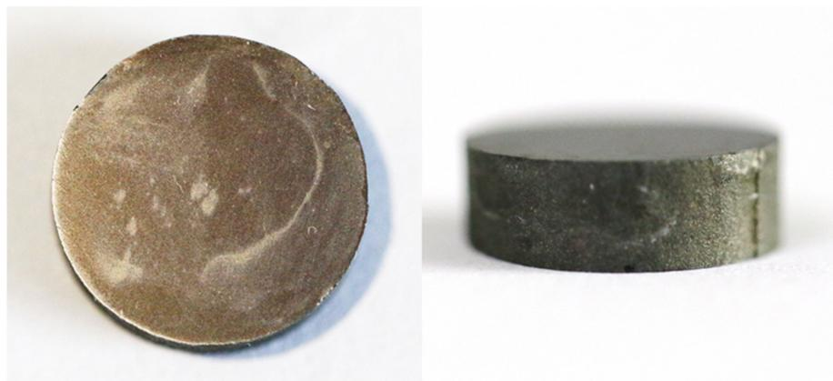
**Figure 1.** Photograph of an Al/Si composite disk sample with 70 vol.% Si.
