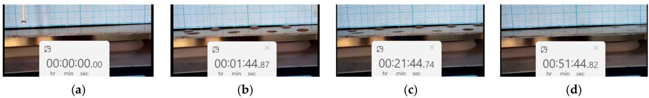
**Figure 7.** Frames from droplet evaporation–corrosion on a steel surface in Test 1, showing that droplet shrinkage occurs with droplet diameter maintained: ( $\varphi = 36.5\%$ ,  $d_0 = 7.2$  mm): (a) blank black steel plate, starting droplet’s deposition; (b) droplet already in position; (c) evaporation evolution after 21 min; (d) end of evaporation and shape formation; (d) bottom-third deposition of the drop,  $\varphi = 43.5\%$ ,  $d_0 = 7.2$  mm.
