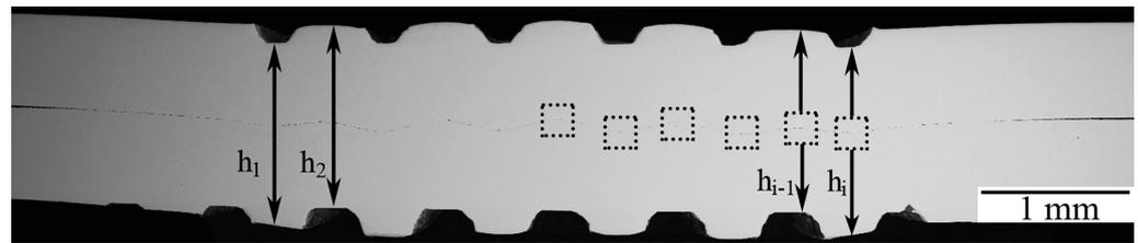
**Figure 3.** A scheme of selection of positions for microstructure imaging and measuring the thickness of a specimen, which was used to evaluate the linear weld density and the normal strain of samples at the same point of a joint.
