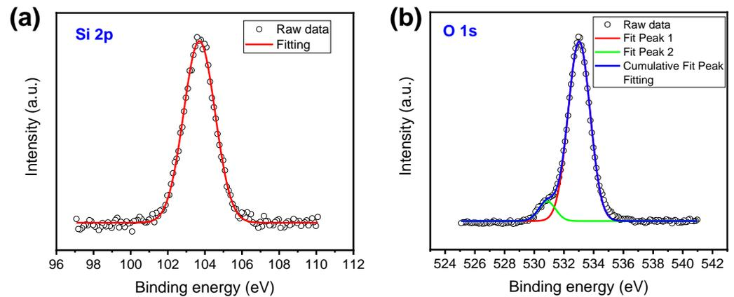
**Figure 2.** The XPS core level spectra of the ALD deposited  $\text{SiO}_x$  film: (a) Si 2p; (b) O 1s.
