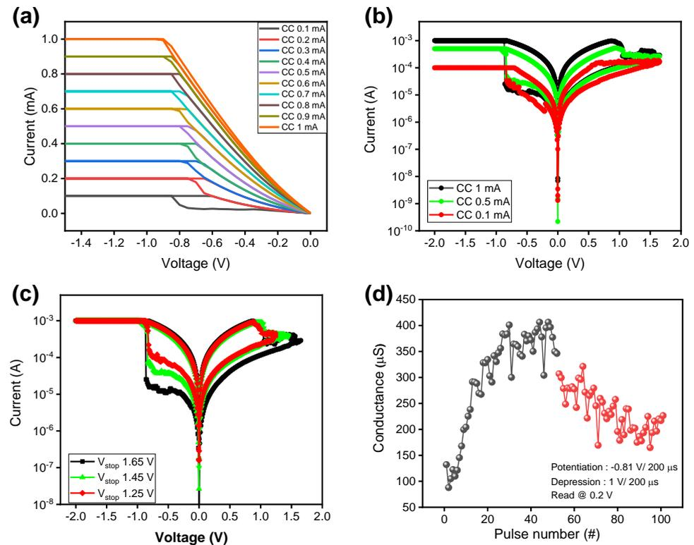
**Figure 4.** The MLC characteristics of the Pt/SiO<sub>x</sub>/Ta<sub>n</sub> RRAM device: (a) plots of the low-resistance current with various compliance currents; (b and c) controlling the bipolar resistive switching via (b) the compliance current and (c) the reset stop voltage; (d) potentiation (black) and depression (red) by the application of negative and positive pulses, respectively.
