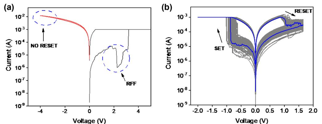
**Figure 3.** The I-V characteristics of the Pt/ $\text{SiO}_x$ /Ta $\text{N}$  RRAM device under (a) positive set and negative reset operation, and (b) negative set and positive reset operation.
