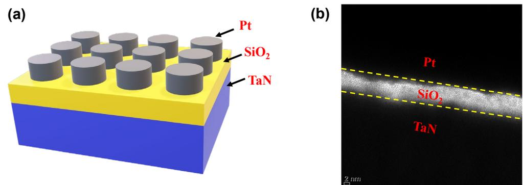
**Figure 1.** A schematic diagram (a) and cross-sectional TEM image (b) of the Pt/SiO<sub>x</sub>/TaN RRAM device.
