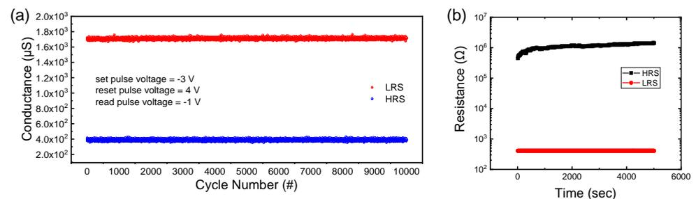
**Figure 5.** (a) Pulse endurance and (b) retention properties of the Pt/SiO<sub>x</sub>/Ta<sub>n</sub> RRAM device.
