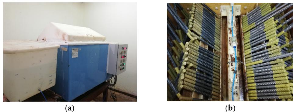
**Figure 3.** (a) View of salt spray chamber in laboratory and (b) view of the tested steel bars in the salt spray chamber.
