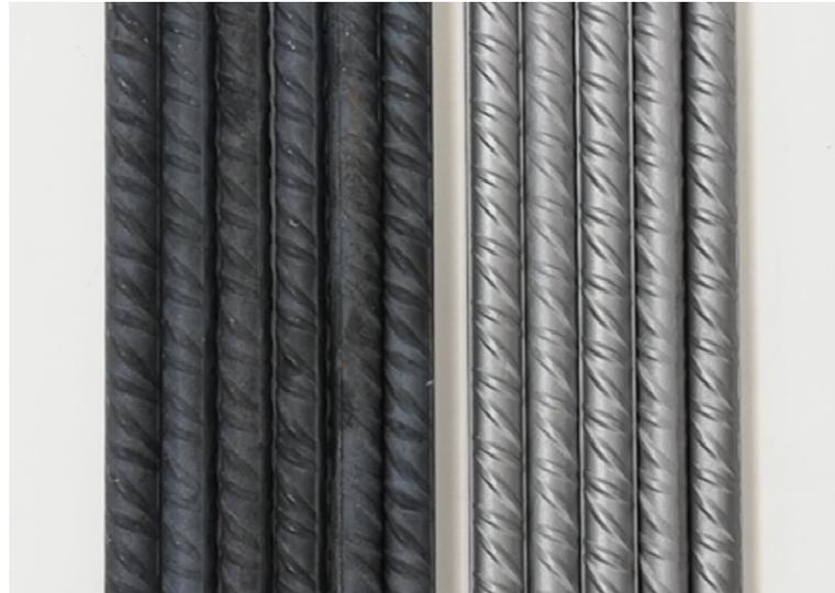
**Figure 2.** Steel (B500c) reinforcing bars before (left) and after (right) shot blasting process.
