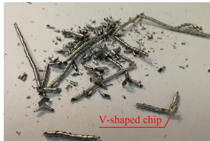
**Figure 5.** The chip morphology after chip-splitting catastrophe: Cutting edge angle  $\theta = 45^\circ$ , Rake angle  $\gamma_0 = -10^\circ$ , Critical cutting thickness  $a_{ce} = 0.0495$  mm.
