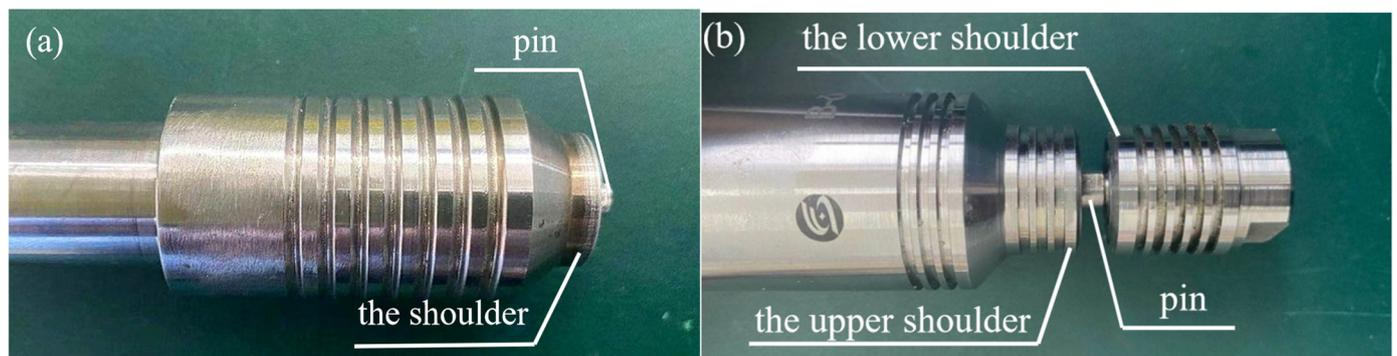
Figure 2. Tool structure: (a) the common FSW tool; (b) BT-FSW tool.
