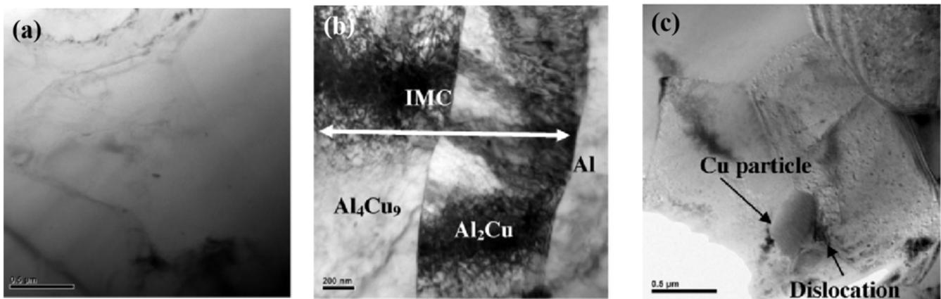
**Figure 17.** TEM investigation of the various regions of the stir zone microstructure at the tool travel speed of 80 mm/min: (a) SZ (Cu side); (b) intermetallic layer; and (c) SZ (Al side) (from ref. [54]).
