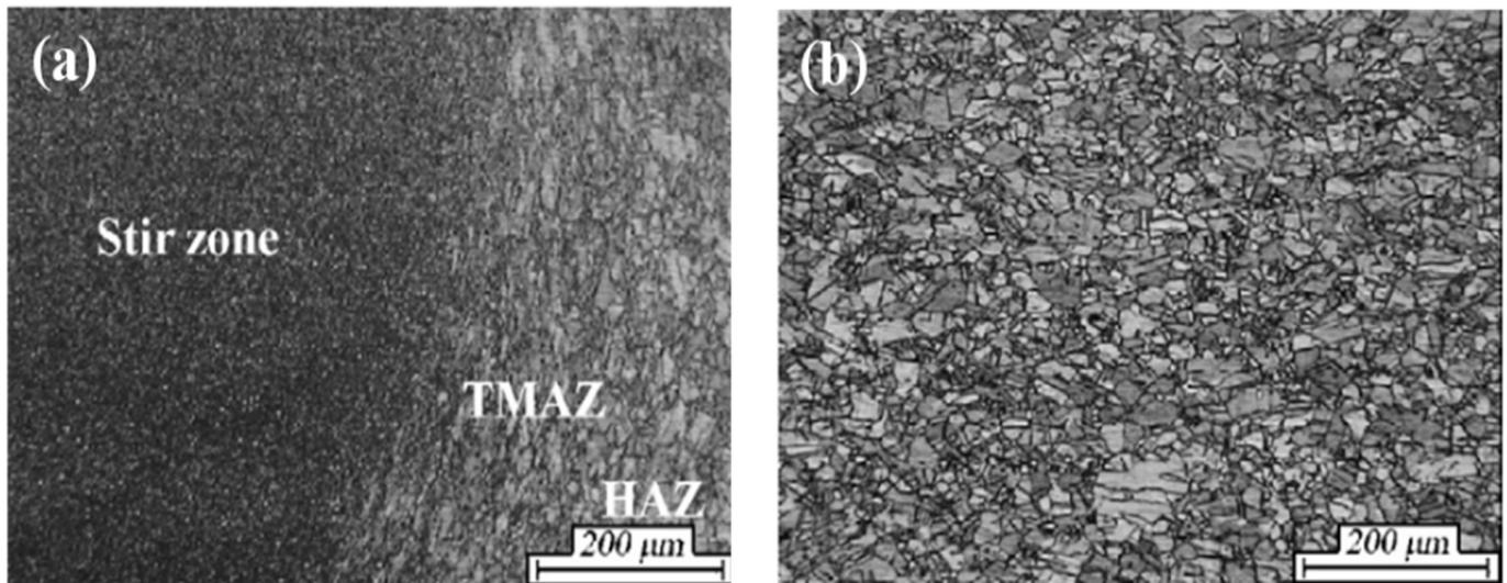
**Figure 11.** (a) Stir zone, TMAZ and HAZ of copper in the advancing side of the joint; (b) HAZ in the copper side (adapted from [71], with permission from Elsevier, 2007).
