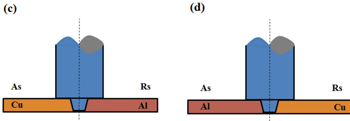
**Figure 6.** Material placement position of (a) Cu on the top; (b) Al on the top; (c) Cu on the AS; (d) Al on the AS.
