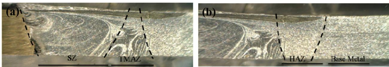
**Figure 13.** Macroscopic morphology of the Cu–Al FSW butt joint (a) SZ and TMAZ; (b) HAZ and base metal (adapted from [42], with permission from Elsevier, 2011).
