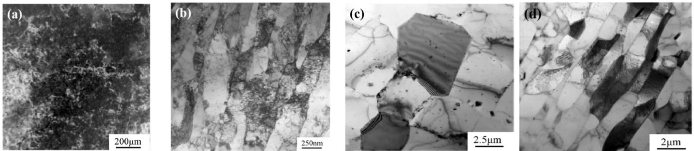
**Figure 14.** (a) TEM bright field of the dislocation organization in the copper base material; (b) bright-field TEM micrograph showing the grain and the dislocation structures in the TMAZ in the copper side, close to the Al/Cu interface; (c) bright field showing the microstructure in the stir zone; (d) bright field of the grain structure in the TMAZ (adapted from [15], with permission from Springer, 2011).
