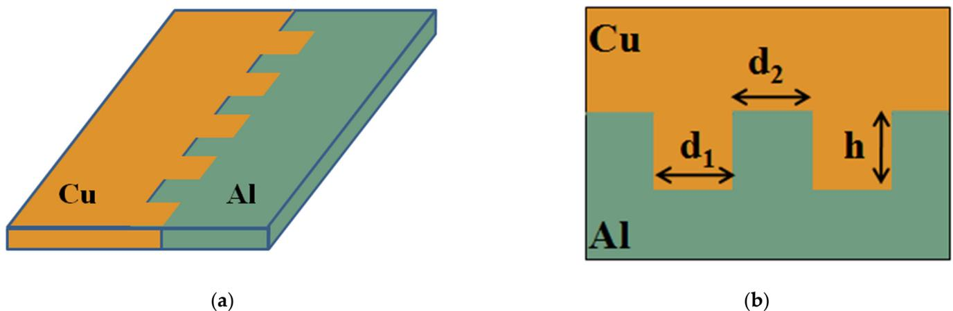
**Figure 20.** (a) schematic diagram of tooth-shaped butt joint; (b) Dimension diagram.
