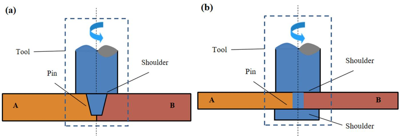
**Figure 1.** Principle of FSW: (a) single-shaft shoulder FSW; (b) bobbin tool FSW.
