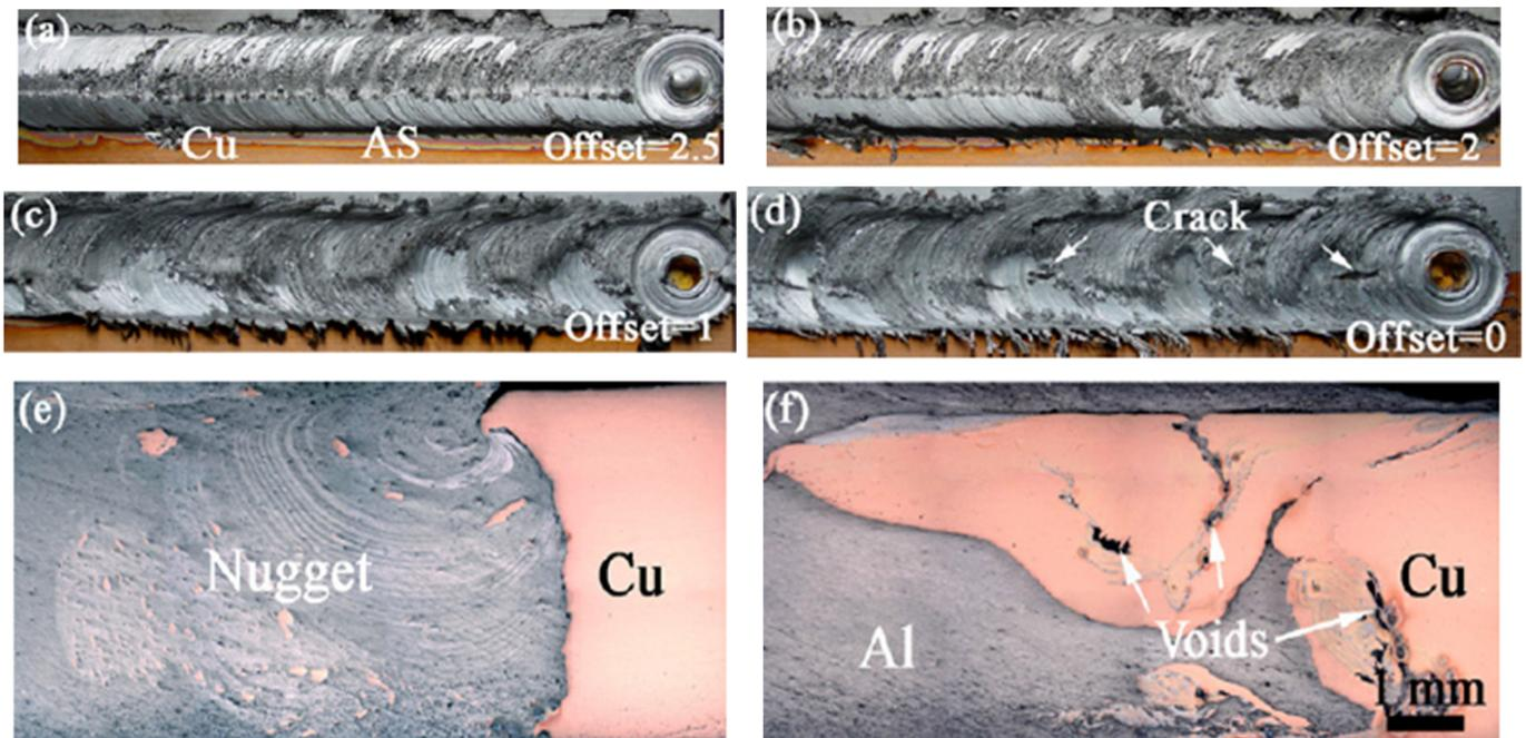
**Figure 9.** Surface morphologies of the FSW Al–Cu joints for pin offsets of (a) 2.5 mm; (b) 2 mm; (c) 1 mm; and (d) 0 mm. Cross-sectional macrostructure of the joints for pin offset of (e) 2.5 mm and (f) 1 mm (adapted from [13], with permission from Elsevier, 2011).
