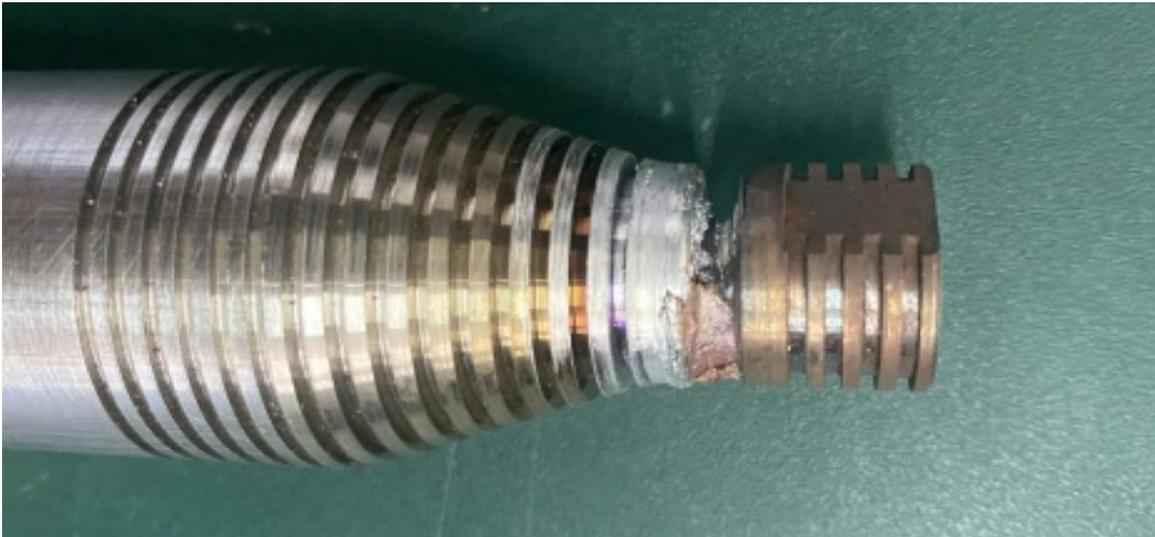
**Figure 5.** The phenomenon of the material adhesion in the tool.
