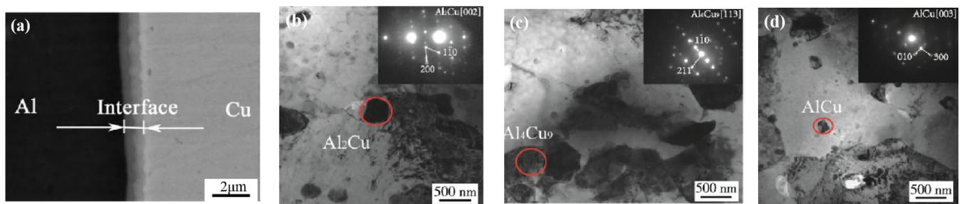
**Figure 16.** (a) Microscope image of a typical IMC (adapted from [3], with permission from Elsevier, 2010); (b) Al<sub>2</sub>Cu<sub>[2]</sub> phase; (c) Al<sub>4</sub>Cu<sub>9[113]</sub> phase; (d) AlCu<sub>[3]</sub> phase (adapted from [62], with permission from CNKI, 2019).
