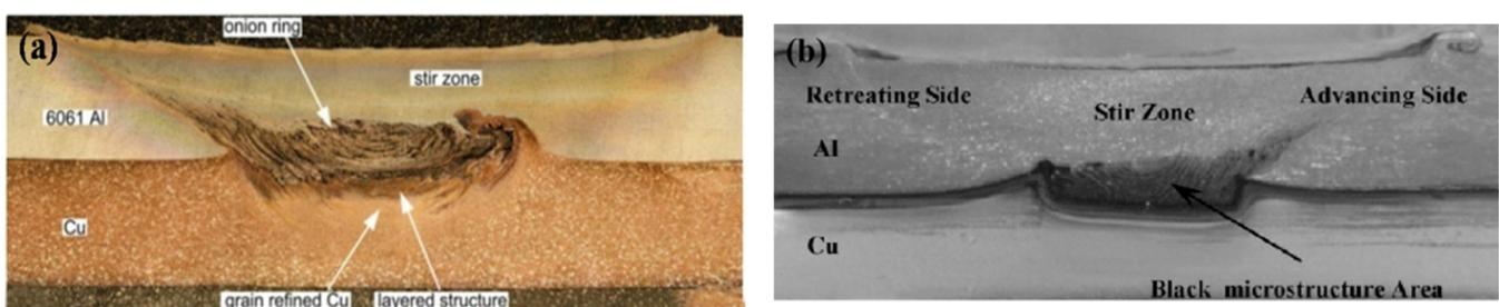
**Figure 10.** Macroscopic morphology of Cu–Al FSW lap joint: (a) (adapted from [72], with permission from Springer, 2011); (b) (adapted from [71], with permission from Elsevier, 2007).
