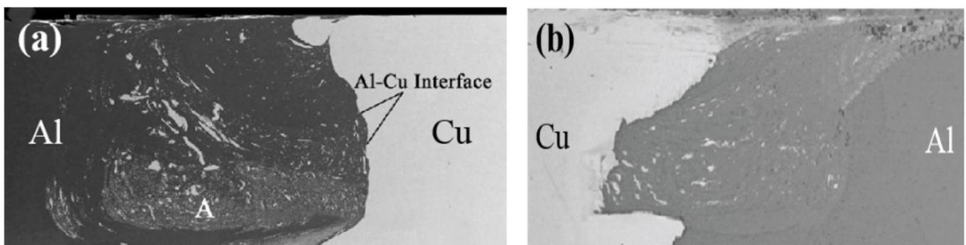
**Figure 15.** (a) SEM backscattered electron images (BEI) of the FSW Al-Cu joint (from ref. [3]); (b) SEM microstructures of the FSW Al-Cu welded joint in NZ (from ref. [62]).
