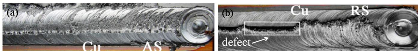
**Figure 7.** Surface morphologies of the FSW Al–Cu joints: (a) Cu plate fixed at AS; (b) Cu plate fixed at RS (adapted from [13], with permission from Elsevier, 2011).
