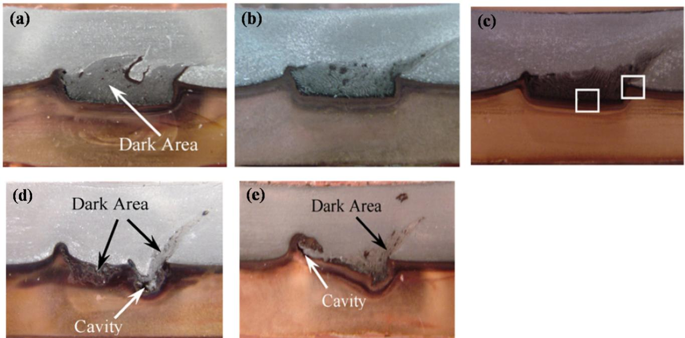
**Figure 12.** Macroscopic overviews of the FSW joint cross sections at the constant tool rotational speed of 1180 rpm and welding speeds of (a) 30, (b) 60, (c) 95, (d) 118 and (e) 190 mm/min (adapted from [6], with permission from Elsevier, 2010).
