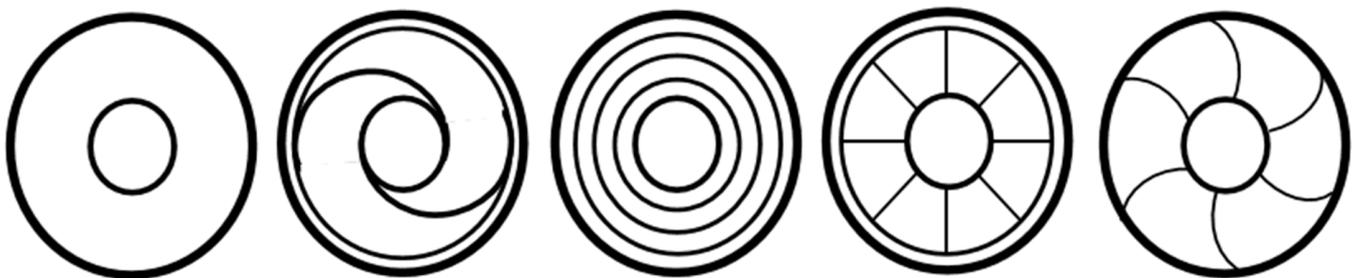
**Figure 3.** Shapes of shoulder suitable for FSW.
