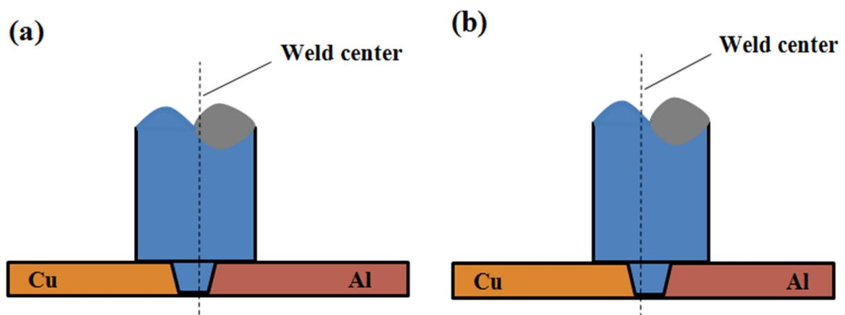
**Figure 8.** The tool bias principle: (a) the tool biased to the Cu side; (b) the tool biased to the Al side.
