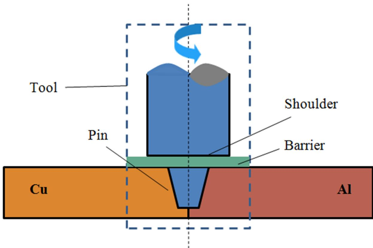
Figure 19. FSBBW schematic diagram.
