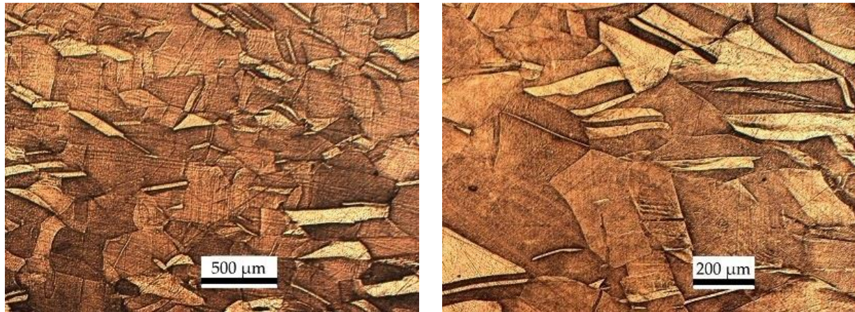
Figure 8. Microstructure of the elastic deformation zone for an impact velocity of 316 m/s.
