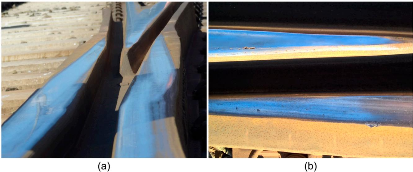
**Figure 1.** Degradation of railway crossing noses: (a) plastic deformation and wear of a manganese crossing nose and (b) material breakouts and spalling/pitting at the crossing nose surface.
