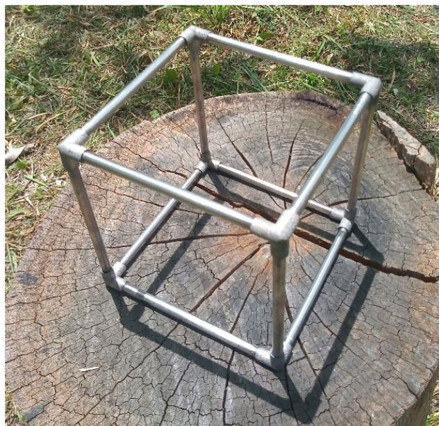
**Figure 3.** Example of the actual CubeSat structure ready for the welds. Each edge measures 100 mm.
