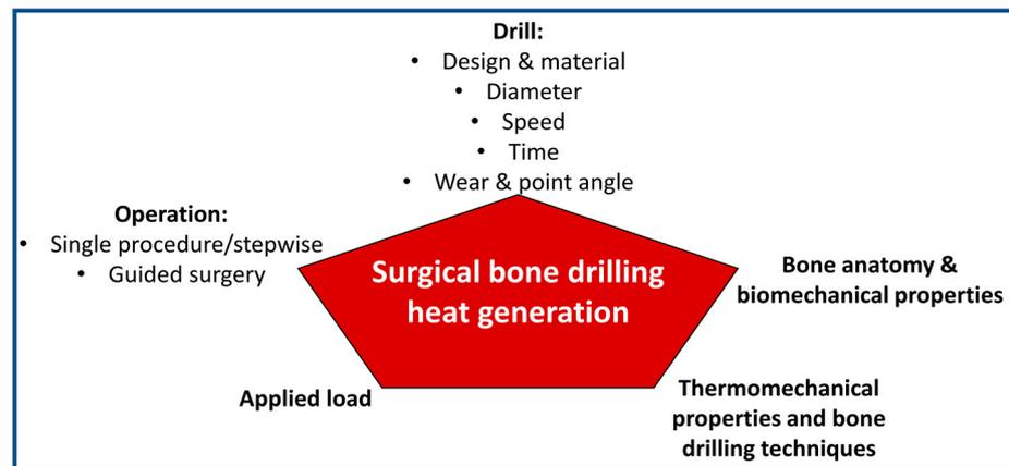
**Figure 1.** Heat generation factors in surgical bone drilling operations.
