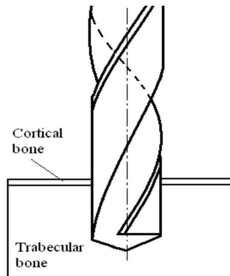
Figure 7. Schematic showing drilling into cortical and trabecular bone [21].
