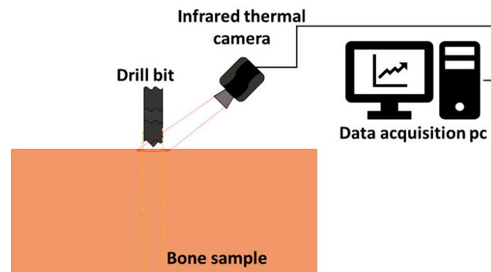
Figure 15. Temperature measurement using a thermal infrared camera [26].
