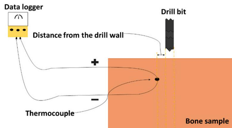
Figure 14. Temperature measurement using a thermocouple [26].
