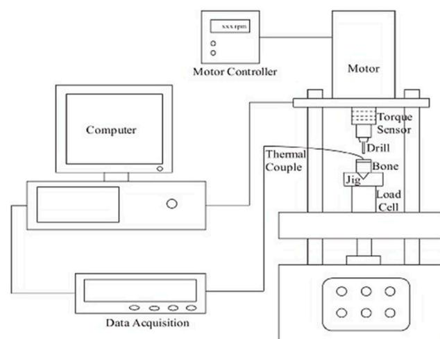
**Figure 5.** Schematic diagram of the bone drilling process [37].
