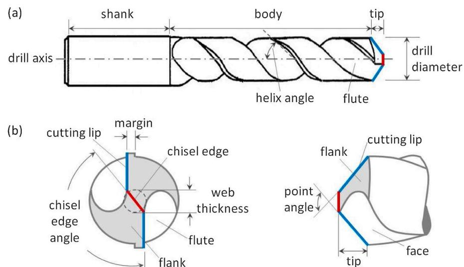
**Figure 11.** Surgical drill bit nomenclature: (a) twist drill bit; (b) axial view of drill bit tip [16].
