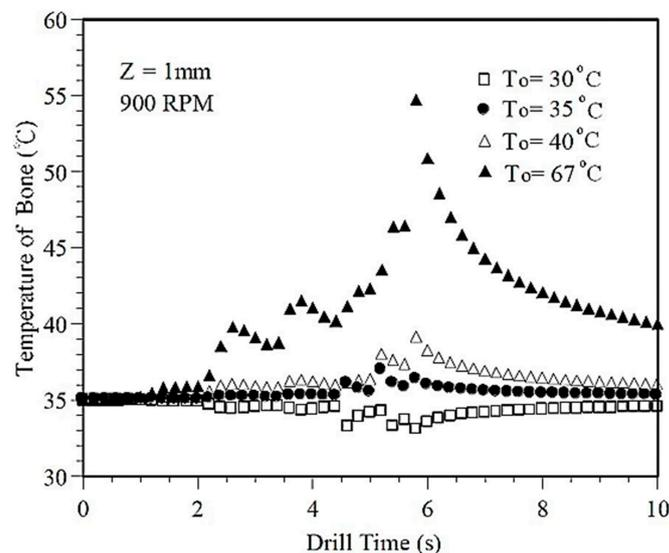
Figure 9. Variation in temperature with the drill time for various initial temperatures [21].
