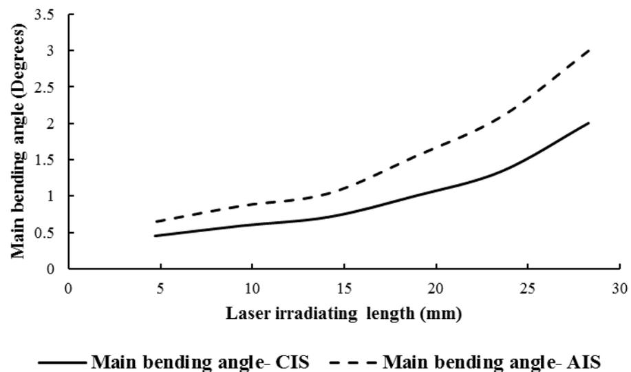
**Figure 4.** The effects of the circular irradiating scheme (CIS) and axial irradiating scheme (AIS) on the main bending angle of the laser-bent tube.
