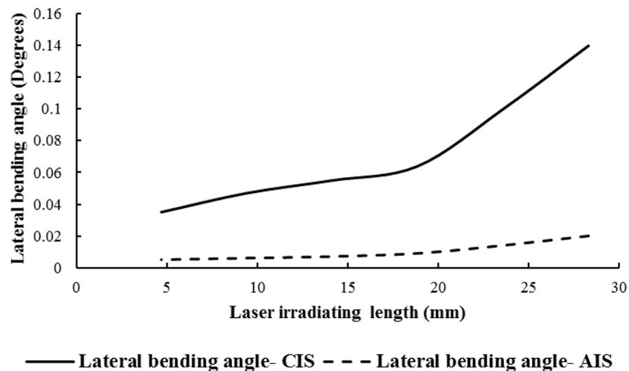
**Figure 5.** The effects of the circular irradiating scheme (CIS) and axial irradiating scheme (AIS) on the lateral bending angle of the laser-bent tube.
