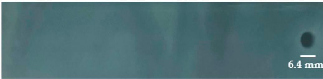
**Figure 13.** Tool 1 trial—X-ray of an AA 6061-T6 aluminum FSW weld.
