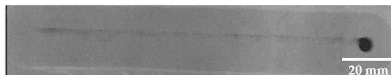
**Figure 10.** X-ray of an AA7075-T6 aluminum FSW weld [117].
