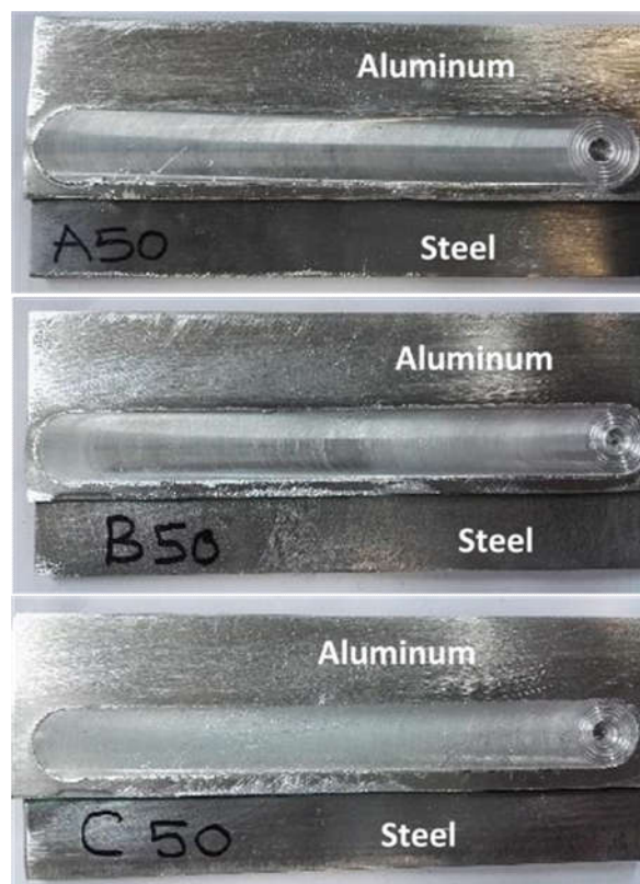
Figure S1. Optical images of typical FSDC processed samples for FH-1 (A50), FM-1 (B50) and FL-1 (C50).
