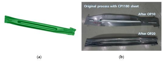
**Figure 11.** Target door impact beam: (a) Modeling of the target door impact beam; (b) Original process (OP10 and OP20) with CP1180 sheet.
