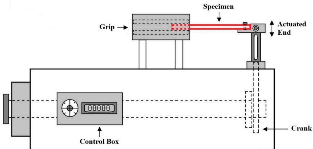
Figure 1. Fatigue bending test rig.
