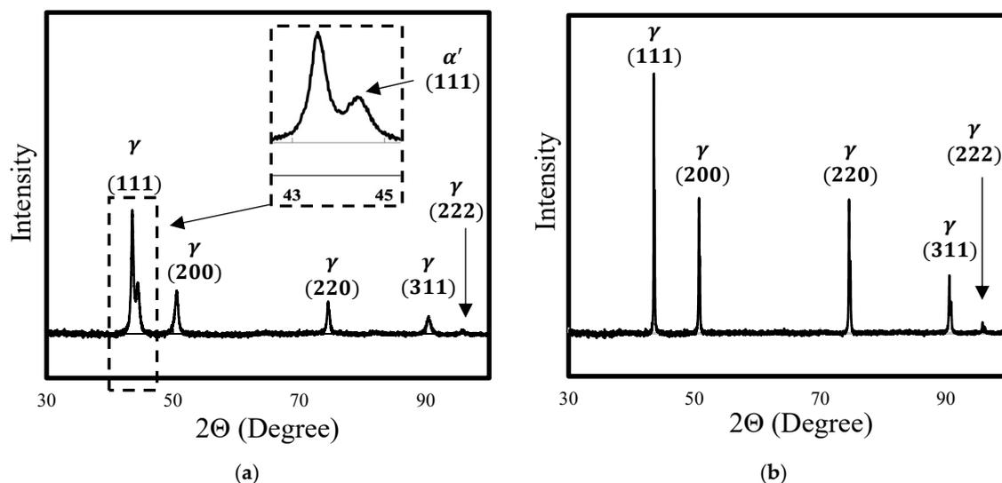
**Figure 8.** XRD profile of the SS316 (a) untreated and (b) heat-treated specimens.
