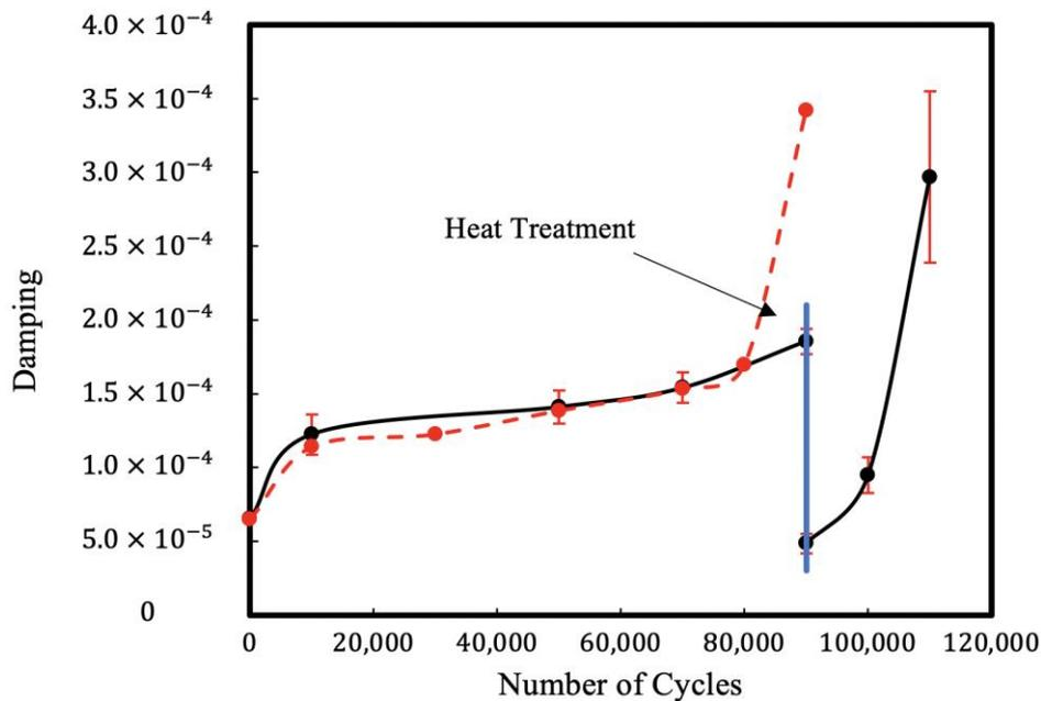
**Figure 7.** Evolution of damping for an SS316 specimen versus the number of cycles with the load frequency of 20 Hz and stress amplitude of 432 MPa halted and heat-treated at the temperature of 600 °C, after crack initiation (90 k). Dashed line results are the damping values of an untreated (as-received) specimen as a benchmark.
