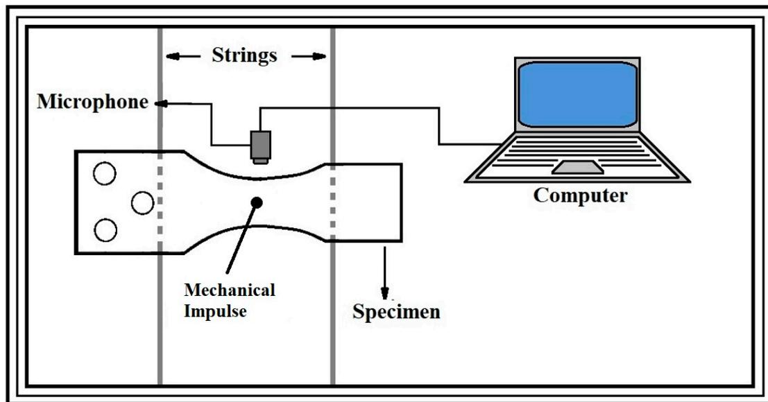
Figure 3. Schematic of the damping measurement setup.
