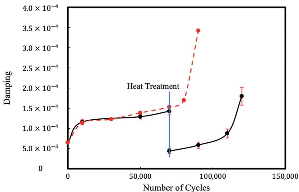
**Figure 6.** Evolution of damping for an SS316 specimen versus the number of cycles with the load frequency of 20 Hz and stress amplitude of 432 MPa halted and heat-treated at the temperature of 600 °C, close to the crack initiation (70 k cycles). Dashed line results are the damping values of an untreated (as-received) specimen as a benchmark.
