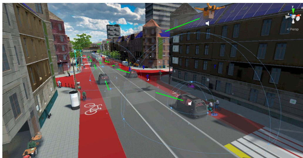
Figure 2. Urban soundscape in the game engine Unity (Source: Marco Weißmann and Dennis Edler, Geomatics Group, Ruhr-University Bochum). The sphere around the vehicle indicates the range of the spatial sound intensity in 3D. The level of loudness decreases with a greater distance from the source (vehicle).
