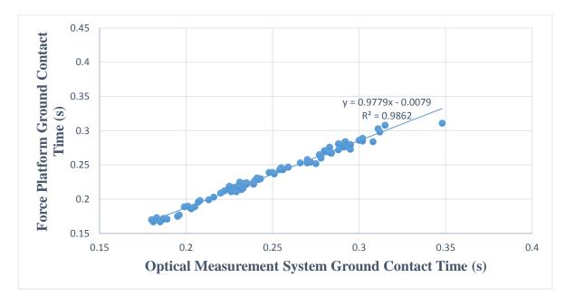
**Figure 2.** Relationship between ground contact time between force platform and optical sensor during drop jump.
