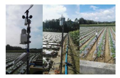
Figure 5. Sensor devices of Caipos.
