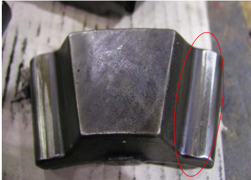
Figure 10. Lower equalizing link from equalized thrust bearing showing mild wear along the contacts.
