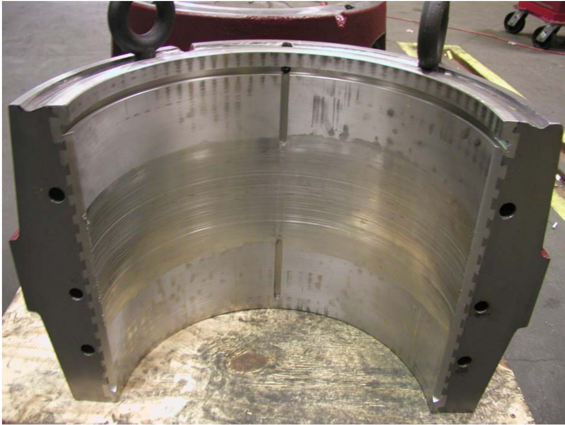
Figure 8. Wiping has covered the axial oil distribution groove on this vertical guide bearing blocking oil flow to the wiped region.
