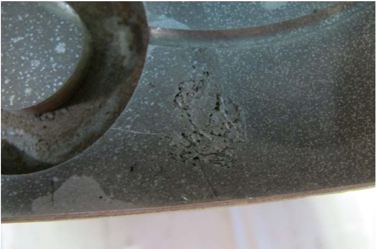
Figure 14. Large region of visual surface porosity with multiple linear indications from static casting observed on a test sample.
