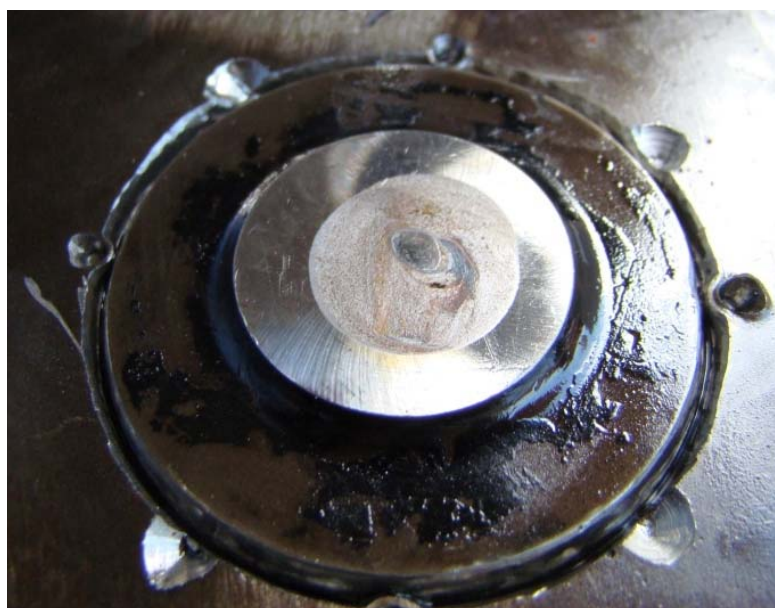
Figure 9. Worn thrust shoe pivot contact showing roughened area (fretting) and material transfer (galling).
