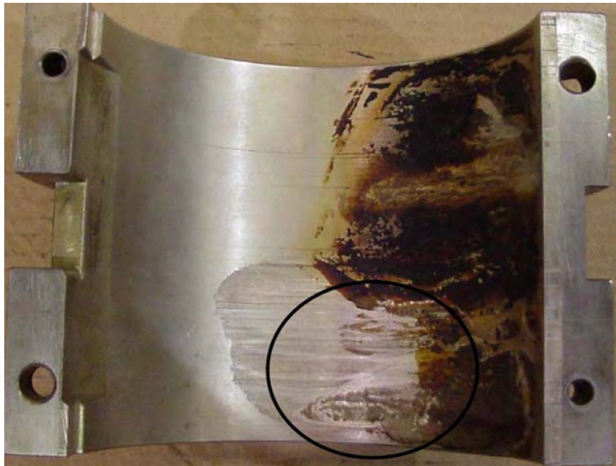
Figure 5. Regions of babbitt material creep in a hot-running region of a cylindrical bearing.
