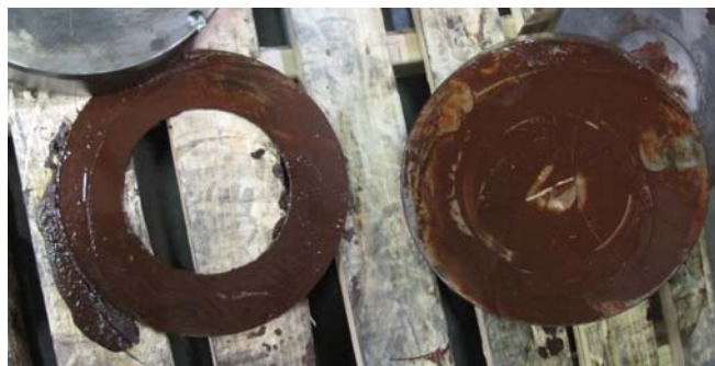
Figure 11. Brown (oily) fretting debris generated between shim ( left ) and pivot support ( right ).
