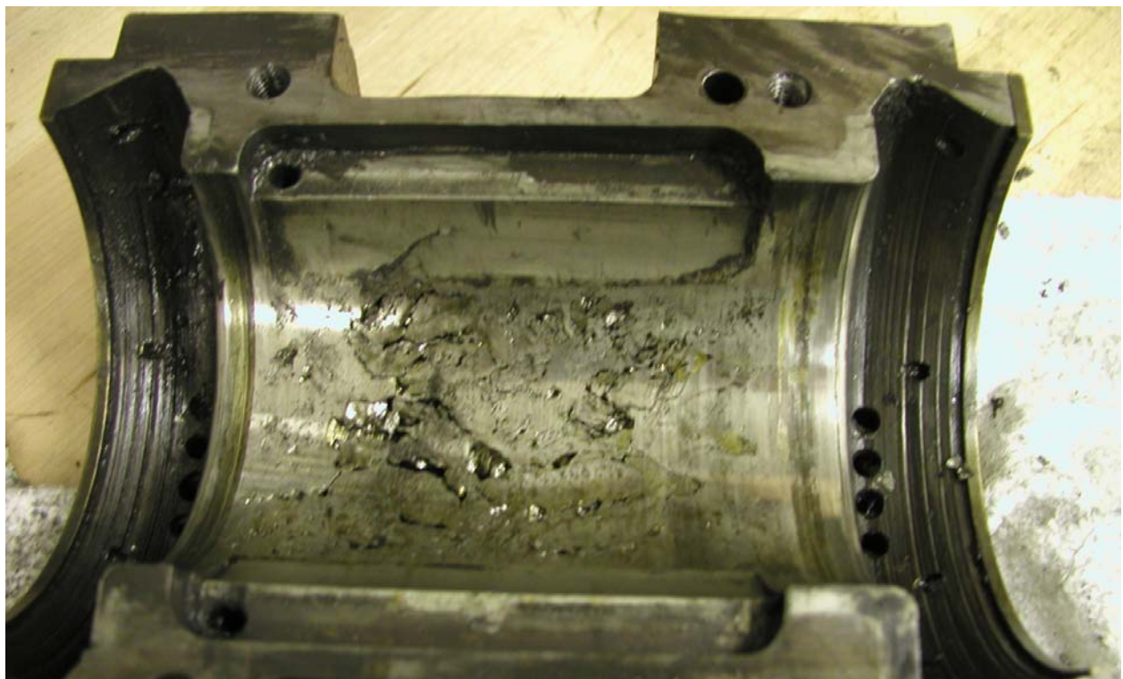
Figure 3. Distributed deep cracking of loaded surface forming an equivalent bulk loss of material.
