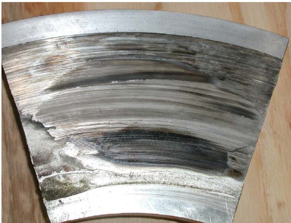
Figure 6. Severe wiping on a thrust shoe (circumferential scratching, narrow lines, also visible).
