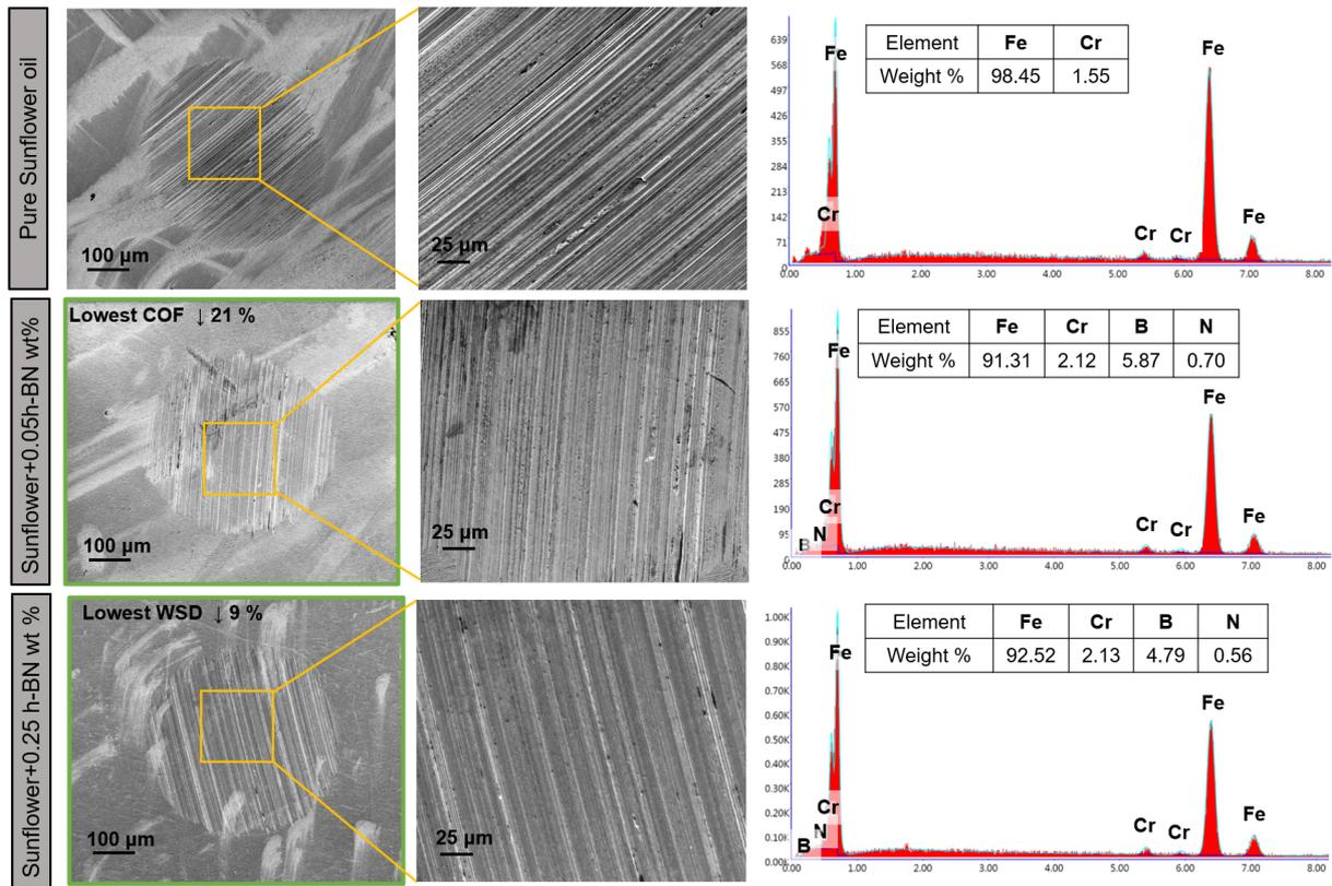
Figure 4. SEM and EDS analysis of the wear scar of the best performing samples of sunflower oil.
