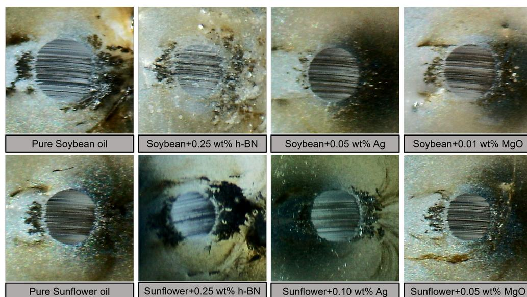
**Figure 6.** Microscopy images of the wear scar captured before cleaning the samples.
