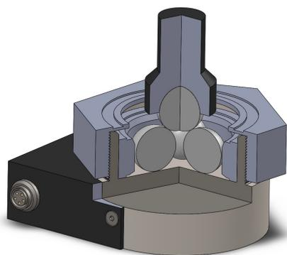
**Figure 1.** Schematic of the Four-ball testing assembly.
