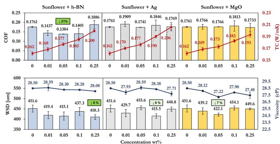
**Figure 2.** Tribological properties of sunflower oil vs. wt% concentration of h-BN, Ag and MgO nanostructures. The error bars represent one standard error (N = 3). The first data point is representative of the base oil.
