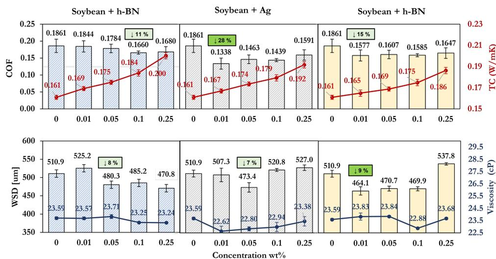
**Figure 3.** Tribological properties of soybean oil vs. wt% concentration of h-BN, Ag and MgO nanostructures. The error bars represent one standard error ( $N = 3$ ). The first data point is representative of the base oil.
