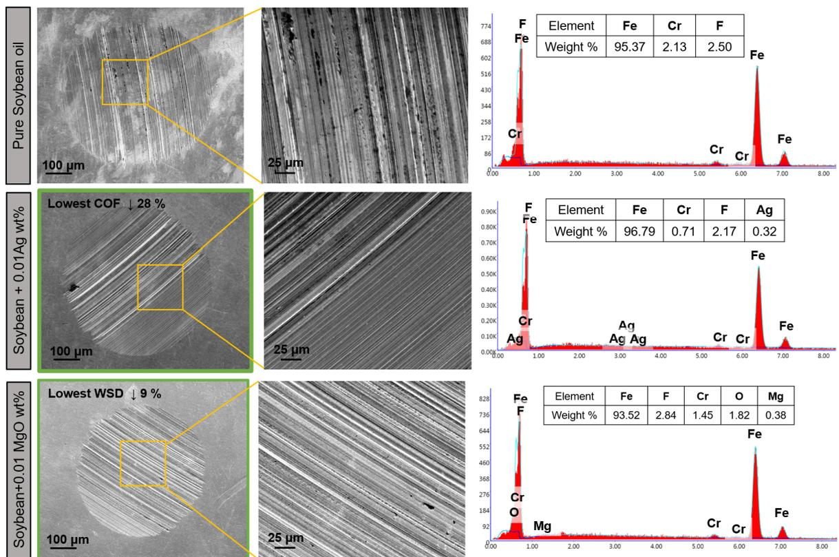
Figure 5. SEM and EDS analysis of the wear scar of the best performing samples of soybean oil.
