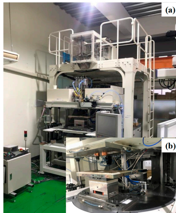
Figure 2. Manufacturing system including the PIG die-casting and hot stamping unit. (a) Overview of the total system, and (b) rotating bed to exchange the die set.
