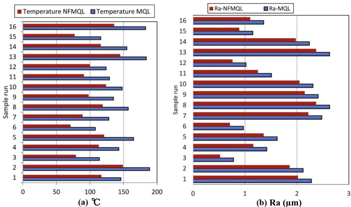
**Figure 1.** Comparison of measurements for MQL and NFMQL (a) Temperature and (b) Surface roughness [27].
