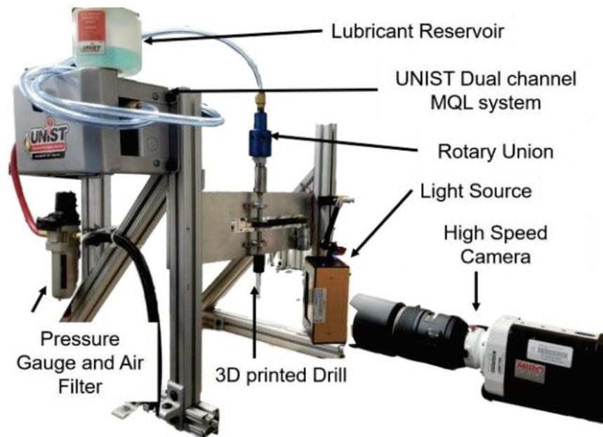
**Figure 4.** Experimental setup for simulating MQL flow in internal channel drill bits [65].
