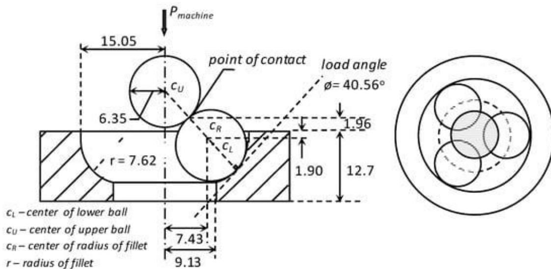
**Figure 3.** Four-ball test setup and the ball configuration and geometry are given in units of mm [33].
