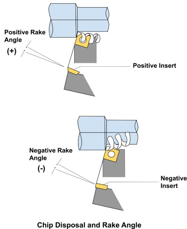
**Figure 2.** Chip Disposal and Rake Angle [36].
