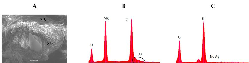
**Figure 4.** SEM image of the aerogel after adenine and colloid and salt deposit and drying (A). (B) and (C) energy dispersive X-Ray spectrometry (EDS) analysis on the focus B and C, respectively.
