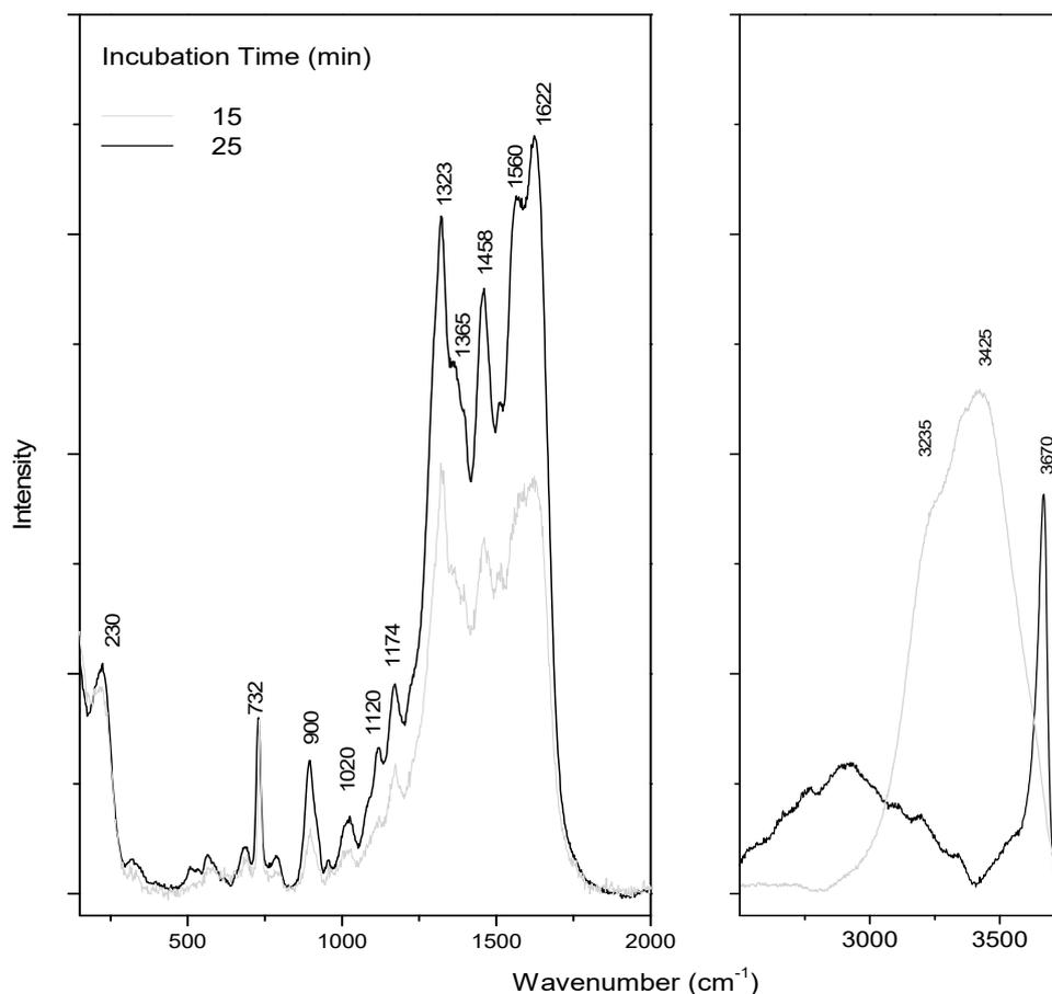
**Figure 2.** SERS adenine spectra as a function of incubation time. A colloid drop was added on dried adenine ( $10\ \mu\text{L}$  of adenine–ethanol solution at  $10^{-3}\ \text{M}$ ) on a glass slide.
