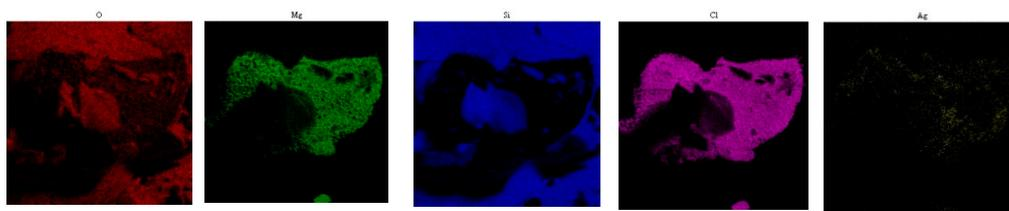
**Figure 5.** Cartographies showing the 2D distribution of some elements characteristic of the colloid and salt (Mg, Cl, Ag) and aerogel (O, Si) (Figure 4A).
