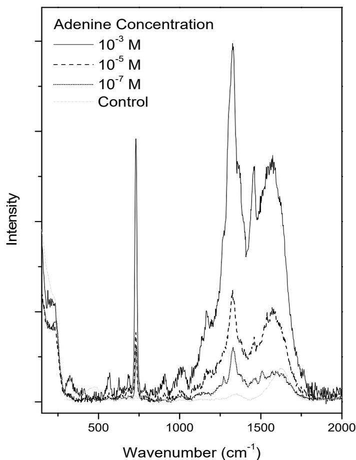
**Figure 3.** SERS adenine spectra as a function of adenine concentration in glass wells after 15 min incubation, with control spectrum (colloid mixture).
