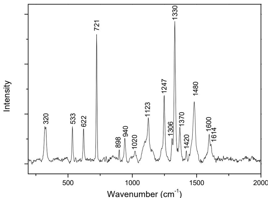
Figure 1. Raman spectrum of adenine powder.
