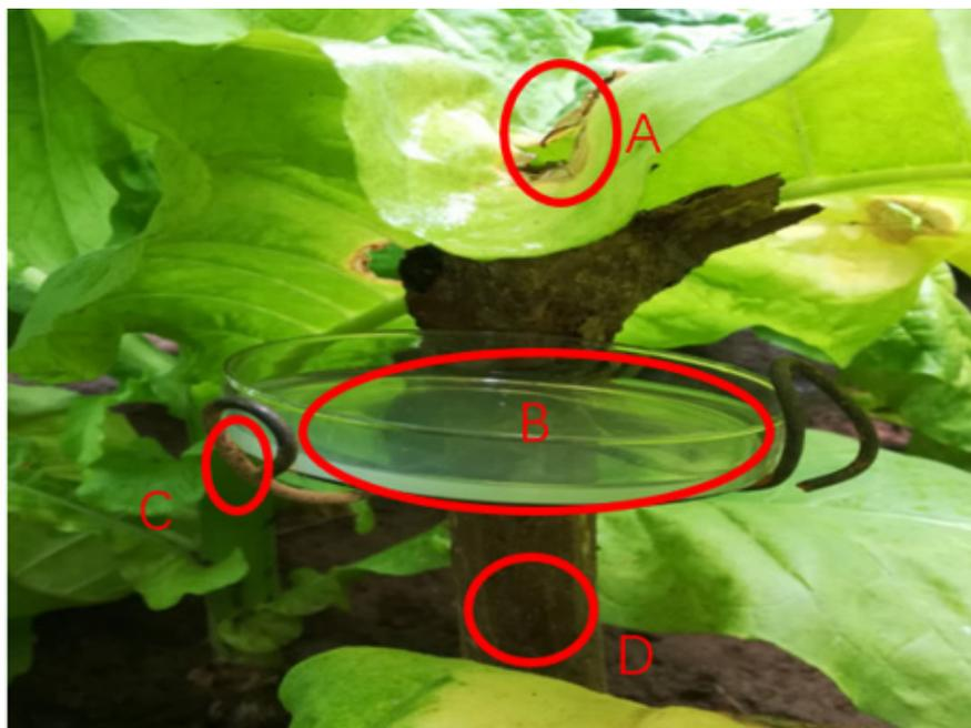
**Figure 2.** A simple device for collecting spores. (A) Diseased leaves in the field. (B) Water agar medium. (C) Fixed rigging. (D) Support tool for adjustment height.
