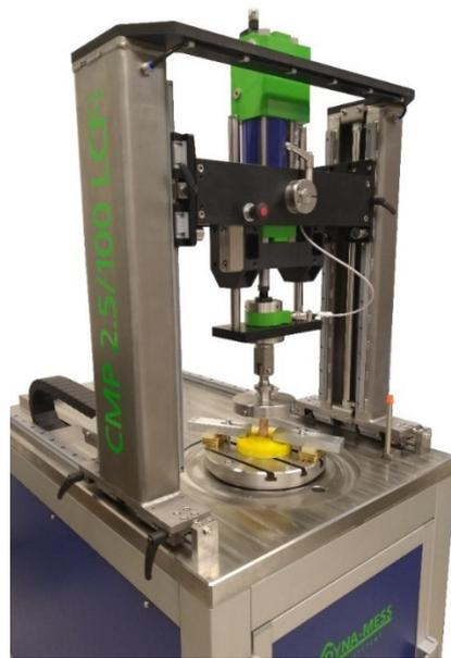
**Figure 3.** DYNA-MESS machine used for fatigue tests of the specimens. The specimen is a porcine bone used for pilot tests.
