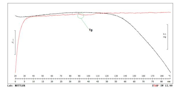
Figure 8. TG-DTA analysis of PMMA.
