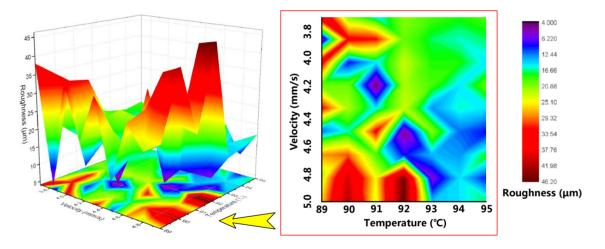
**Figure 9.** Effect of thermal engraving velocity and temperature on roughness in a 100  $\mu$ m width microchannel.
