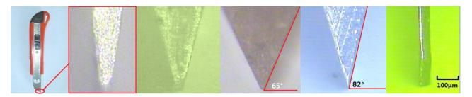
Figure 5. Micrograph of different shapes of the engraving microscriber.
