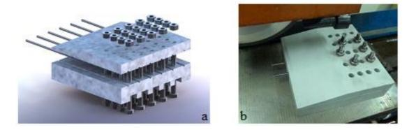
**Figure 3.** The customized fixture. (**a**) Exploded diagram of the fixture design; (**b**) Fixed tungsten steel rods prepared for the precision grinding process.
