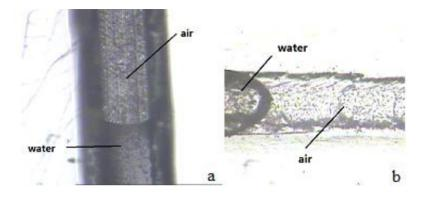
**Figure 13.** Surface wettability of microchannels with different roughness. (**a**) Surface wettability of a smooth microchannel; (**b**) Surface wettability of a rough microchannels.
