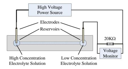
Figure 14. Measurement of the electro-osmotic flow rate using the current monitoring method.
