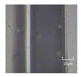
Figure 12. A 30 µm width rectangle microchannel.
