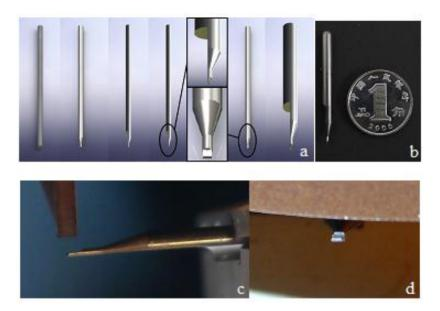
**Figure 2.** Fabricating of a rectangle microscriber. (**a**) Fabrication process of a rectangle microscriber; (**b**) A rectangle microscriber after fabrication; (**c**) A rectangle microscriber prepared for the precision grinding process during the fabrication step; (**d**) A rectangle microscriber prepared for the precision grinding process during the last fabrication step.
