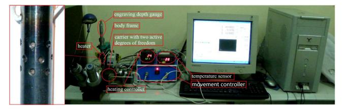
Figure 1. The composition of the equipment.
