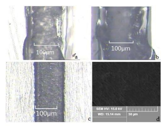
Figure 10. Microchannels under different fabrication conditions. (a) A microchannel fabricated without heating; (b) A microchannel fabricated at 133  $^{\circ}$ C; (c) A smooth microchannel fabricated with an engraving velocity of 4.2 mm/s and a temperature of 93  $^{\circ}$ C; (d) Details of the bottom of the smooth microchannel.
