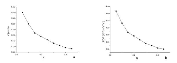
**Figure 15.** Electro-osmotic flow (EOF) characteristic changes with roughness for a 100  $\mu$ m microchannel in a 300 V/cm electric field. (**a**) EOF velocity changes with different roughness; (**b**) EOF changes with different roughness.
